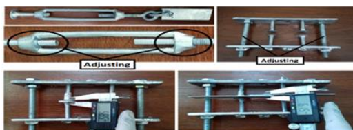
Figure 5: The Instruments that use to adjust the thickness of adhesive material in specimens
