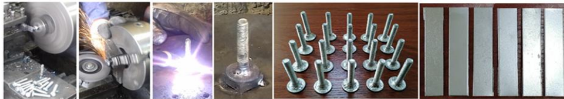
Figure 4: Manufacture and prepare the adherent
