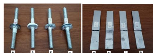
Figure 6: The specimens of butt-off and single lap joint
