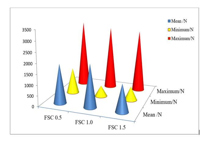
Figure (1) The relation between mean, minimum, and maximum value of FSC restoration with three finish line depth Table (3) illustrate all statistical calculation and it shows that almost the pattern of variation will be observed even when median value is considered. The result was quite Close for all the three group of experiment. In fact, the range of variation between all groups was only 731.5 & 731.38 for both median and mean values respectively.
