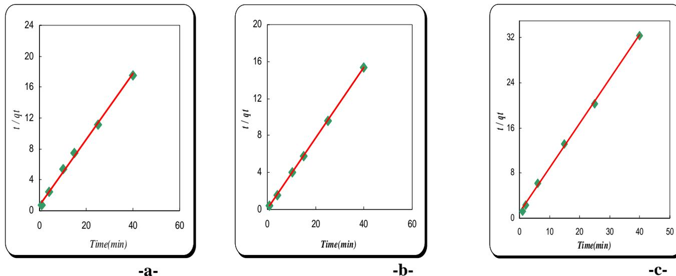
**Figure (5): The applicability of the second order kinetic model to a) Congo red, b) Eosin B and c) Neutral red adsorption on kaolin.**
