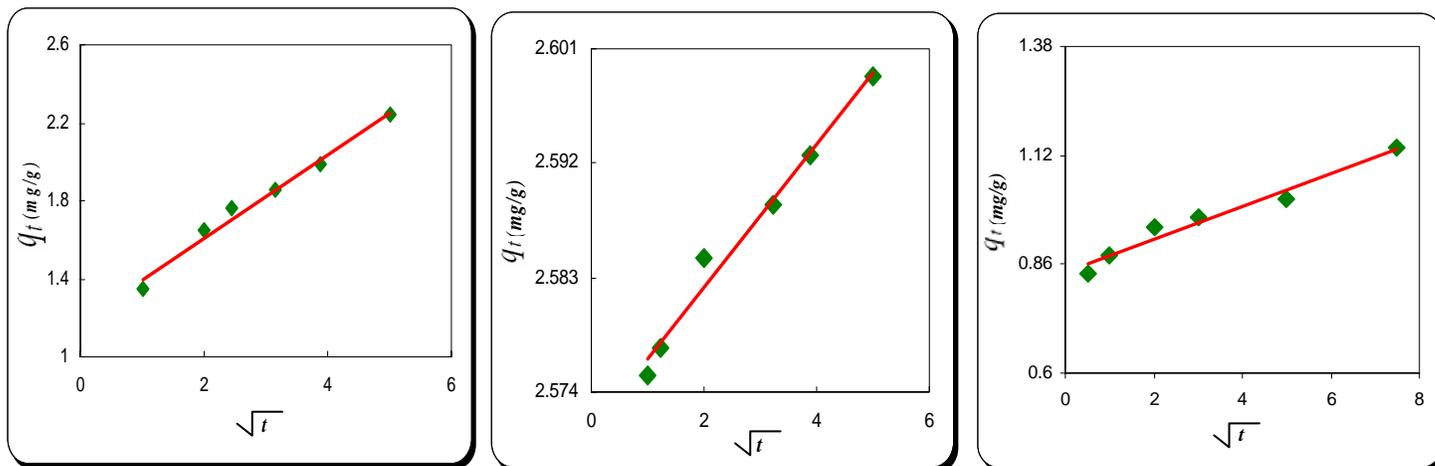
**Figure (6): a) Congo red, b) Eosin B and c) Neutral red uptake by kaolin according to the intraparticle diffusion model.**
