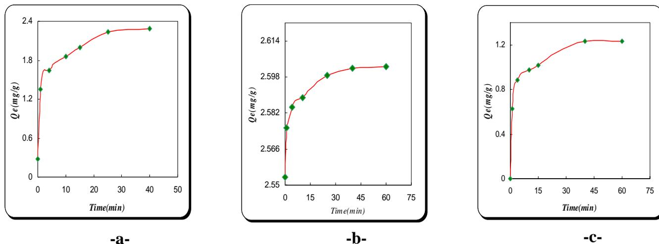
**Figure (1) a- Adsorption kinetics of a- Congo red b- Eosin B c- Neutral red on Kaolin**
