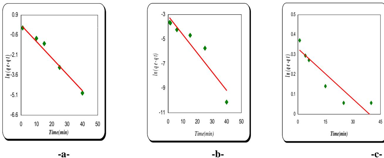
**Figure (4): The applicability of the first order kinetic model to a) Congo red, b) Eosin B and c) Neutral red adsorption on kaolin.**
