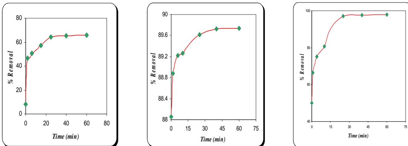
**Figure (3) : Effect of contact time on the removal of a) Congo red b) Eosin B and c) Neutral red by kaolin**
