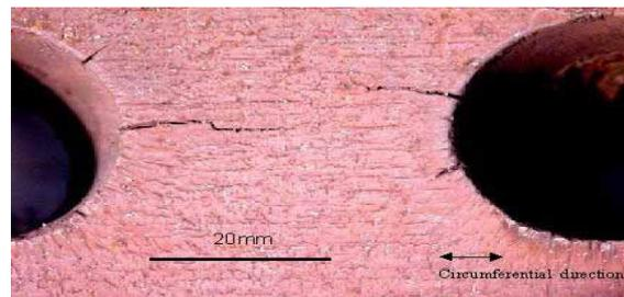
Fig.1 crack due to high thermal stresses (Price, et al 2004)
