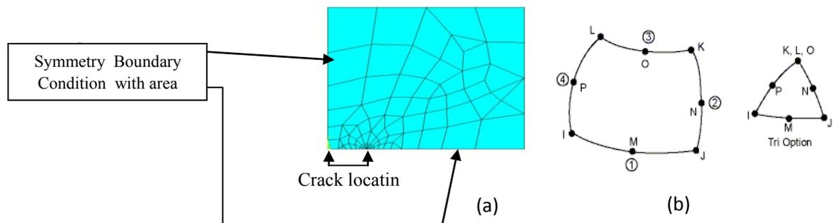
Fig.4 Finite element mesh and element shape
