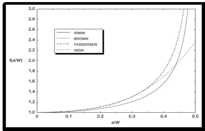
Fig.3 Comparison of correction factor for the center crack (Janssen, et al 2004)
