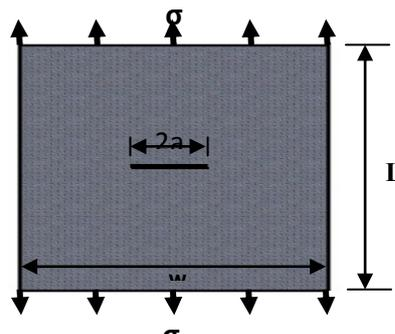
Fig.2 Plate with central crack (Shukla 2005)
