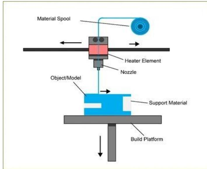
Fig.2. Fused Deposition Modeling (FDM)
