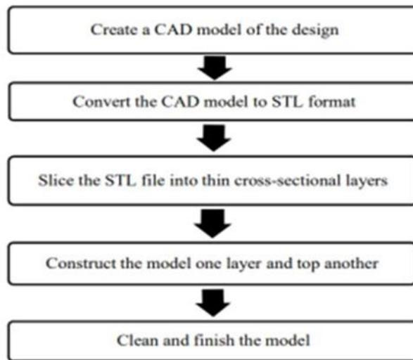
Fig.1.steps of rapid prototyping
