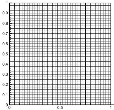
Fig 2 Uniform grid distribution (41×41) for the rectangular enclosure, AR=1.
