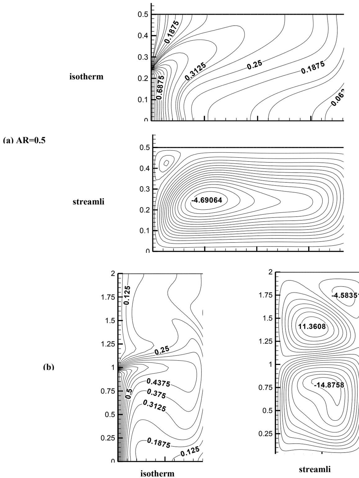
Fig 9 isotherms and streamlines contours of partial heated left wall (lower position), right cold wall and adiabatic top and bottom walls inside rectangular enclosure (a) AR=0.5, (b) AR=2, and Ra=10<sup>5</sup>.
