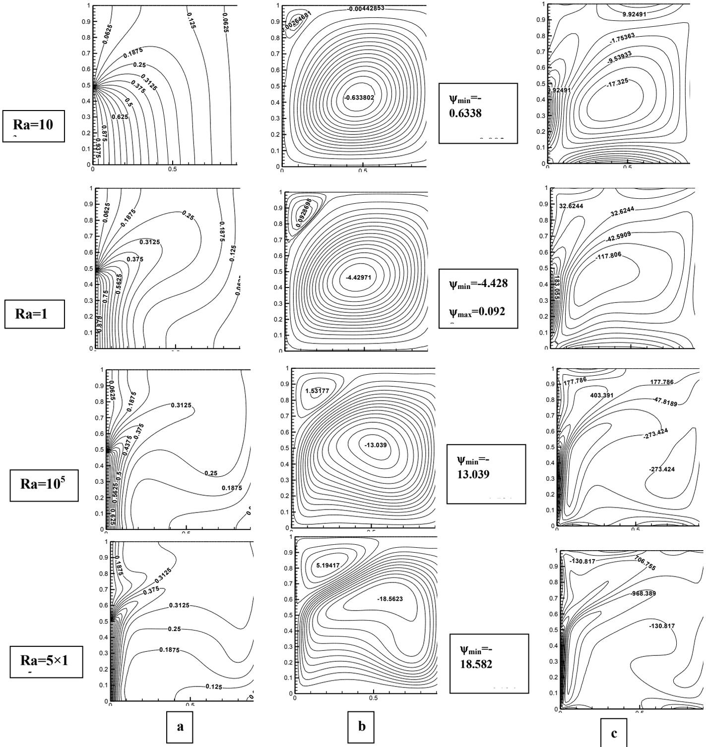
Fig 6 (a)Isotherms; (b)streamlines; (c) vorticity contours of partial heated left wall (lower position), right cold wall and adiabatic top and bottom walls inside rectangular enclosure
