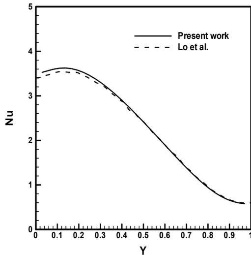
Fig 4 show comparison between present work and Lo et al. for variation Nu at  $Ra=10^4$ .
