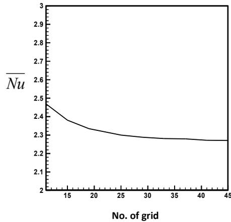
Fig 3 Effect of number of grid on average Nusselt number for Ra=10<sup>4</sup>, AR=1.
