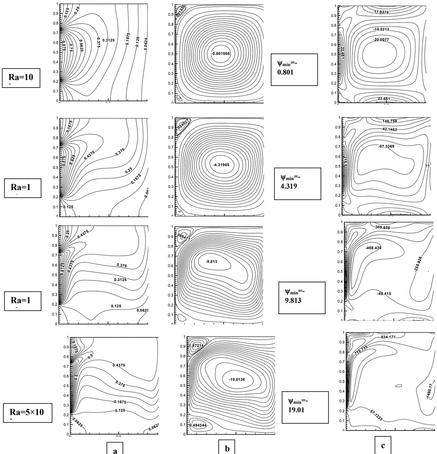
Fig 7 (a)Isotherms; (b)streamlines; (c)vorticity contours of partial heated left wall (center position), right cold wall and adiabatic top and bottom walls inside rectangular enclosure
