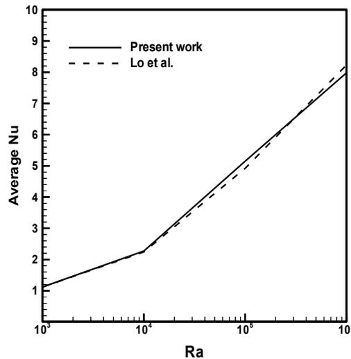
Fig 5 show comparison between present work and Lo et al. for relation between  $Nu$  and  $Ra$ .
