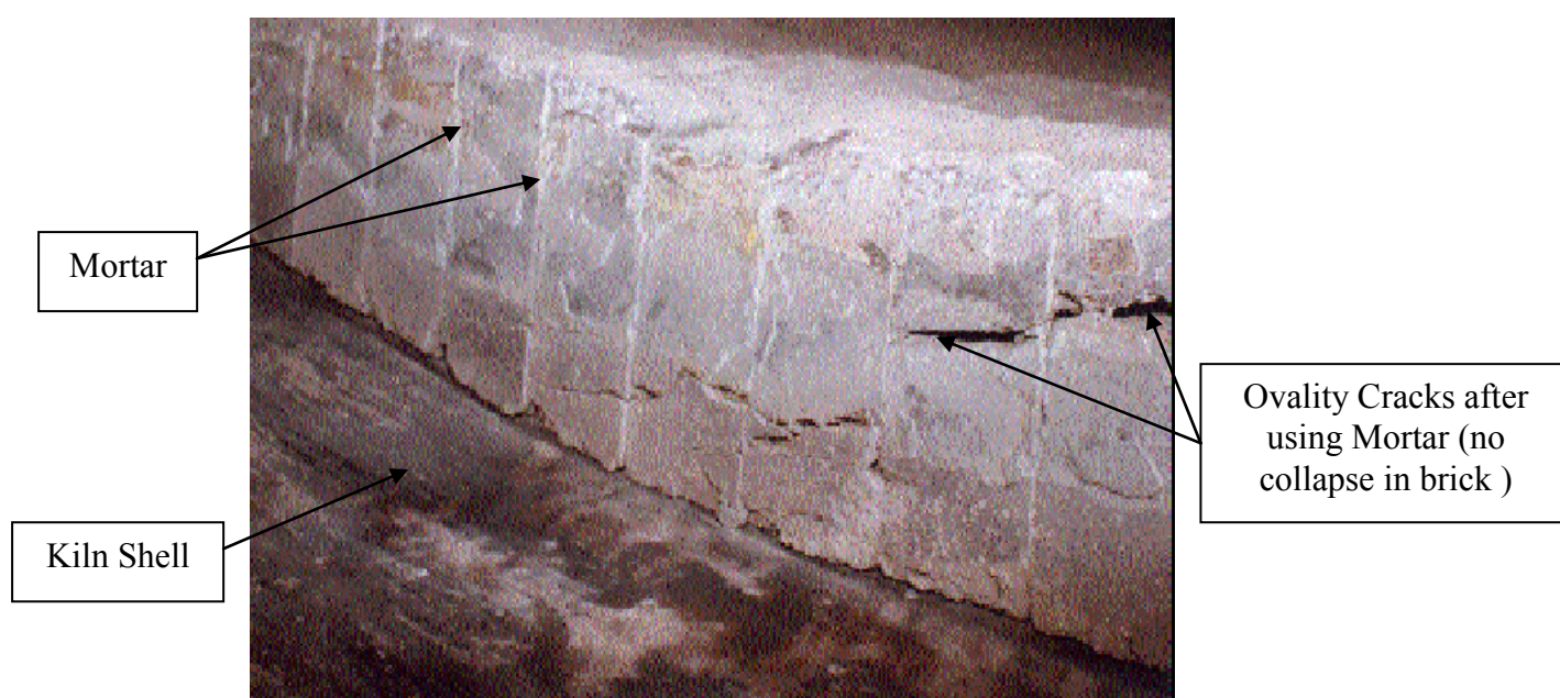
Fig 25 :Using of mortar between bricks to improve its resistance due to Ovality(Resco line Vol.2 2001).
