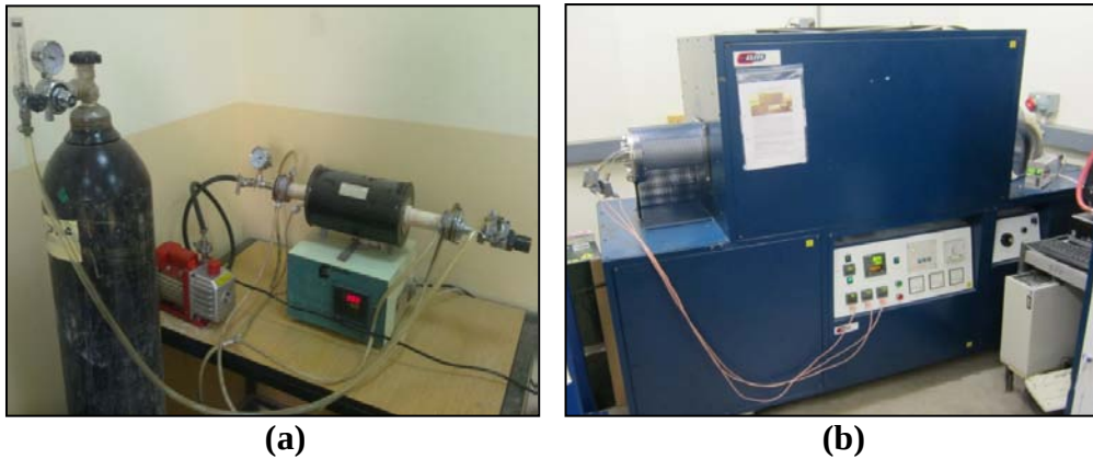
Figure 2: Vacuum tube furnace that is used in the, (a) first calcination condition and (b) second calcination condition.
