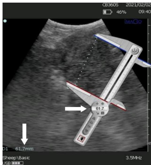
Figure 1: Calibration of the Screen Caliper software through an image of the ultrasonic device with known distances in millimeters.
