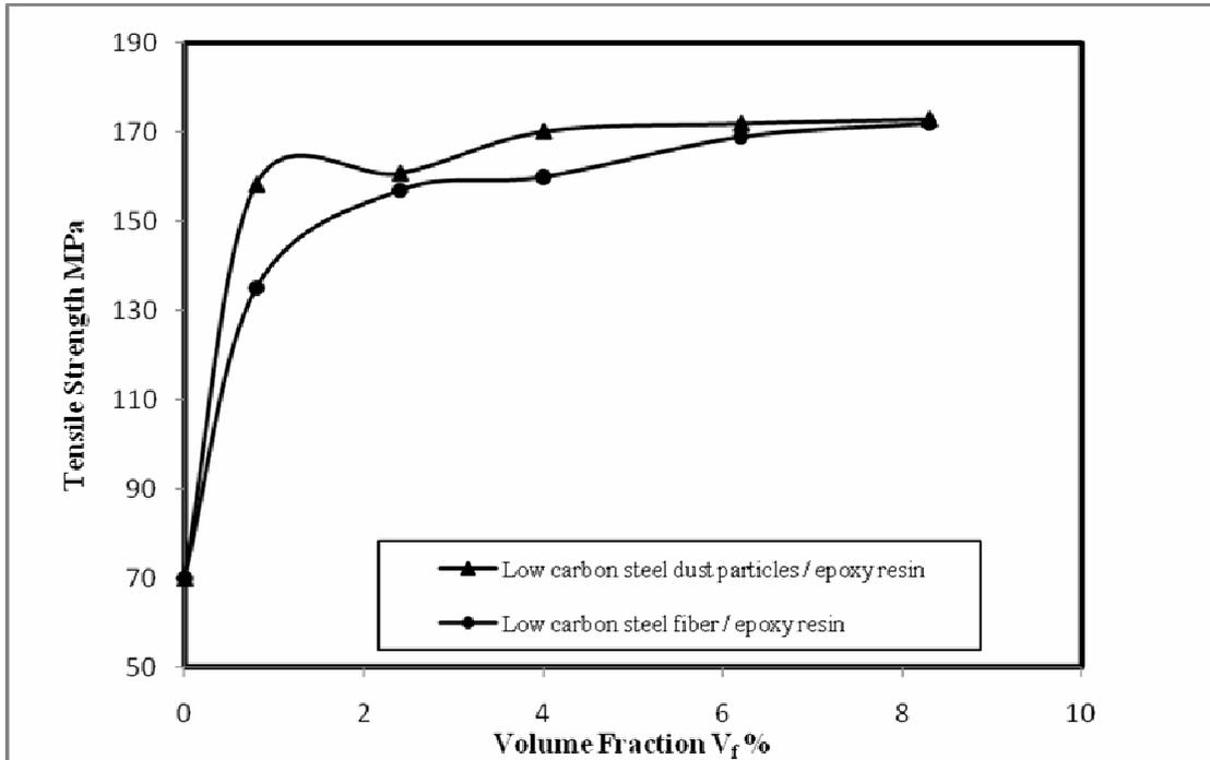
Figure (5) Tensile strength of low carbon steel (fiber and dust particles) / epoxy resin composite
