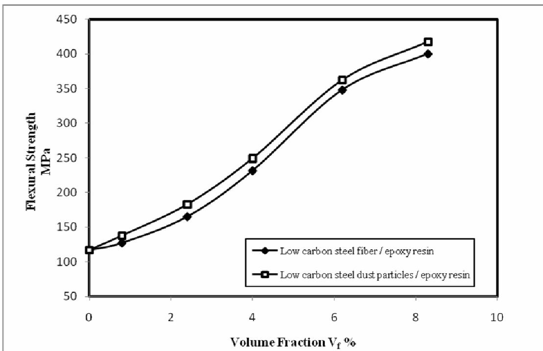
Figure (6) Flexural strength of low carbon steel (fiber and dust particles) / epoxy resin composite
