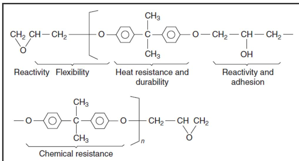
Figure 1 The structure and properties of an epoxy resin (Petrie, E. M, 2006)
