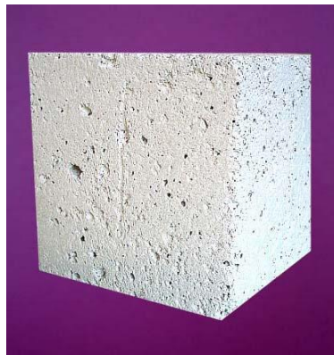
Fig 4: Sample of thermostone ( 100 \times 100 \times 100 ) mm for compression test
