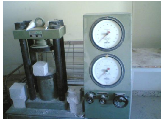
Fig 4: Sample of thermostone ( 100 \times 100 \times 100 ) mm for compression test
