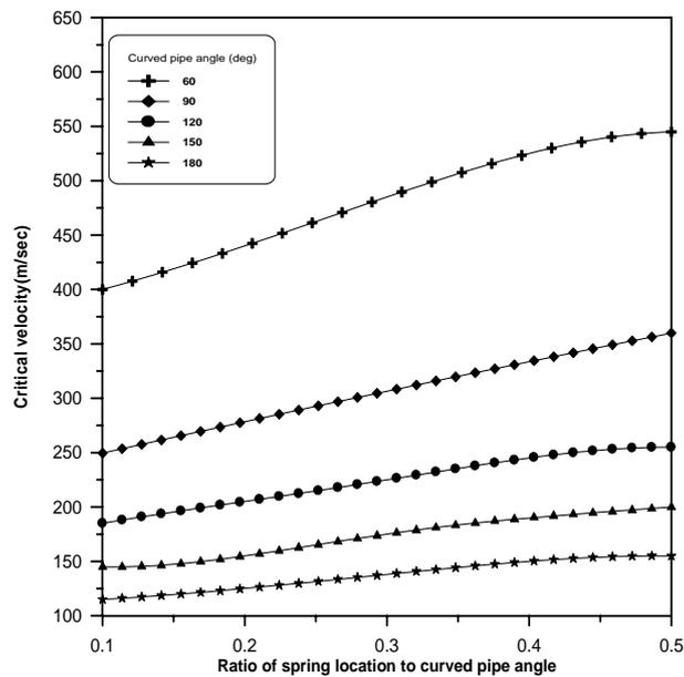
**Fig.(7): Effect the location of spring at curved pipe on the critical velocity with varying curved pipe angle**
