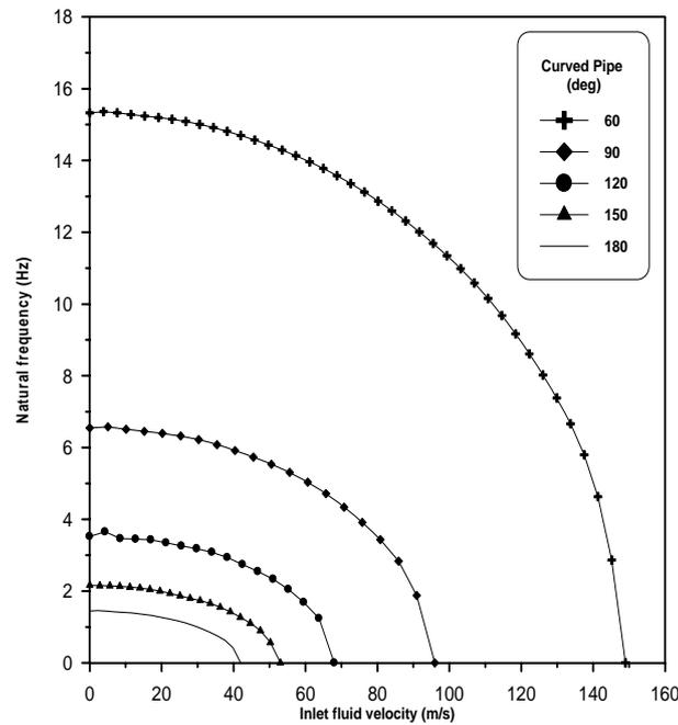
**Fig.(6): Effect the inlet fluid velocity on the natural frequency with different Curved angle**
