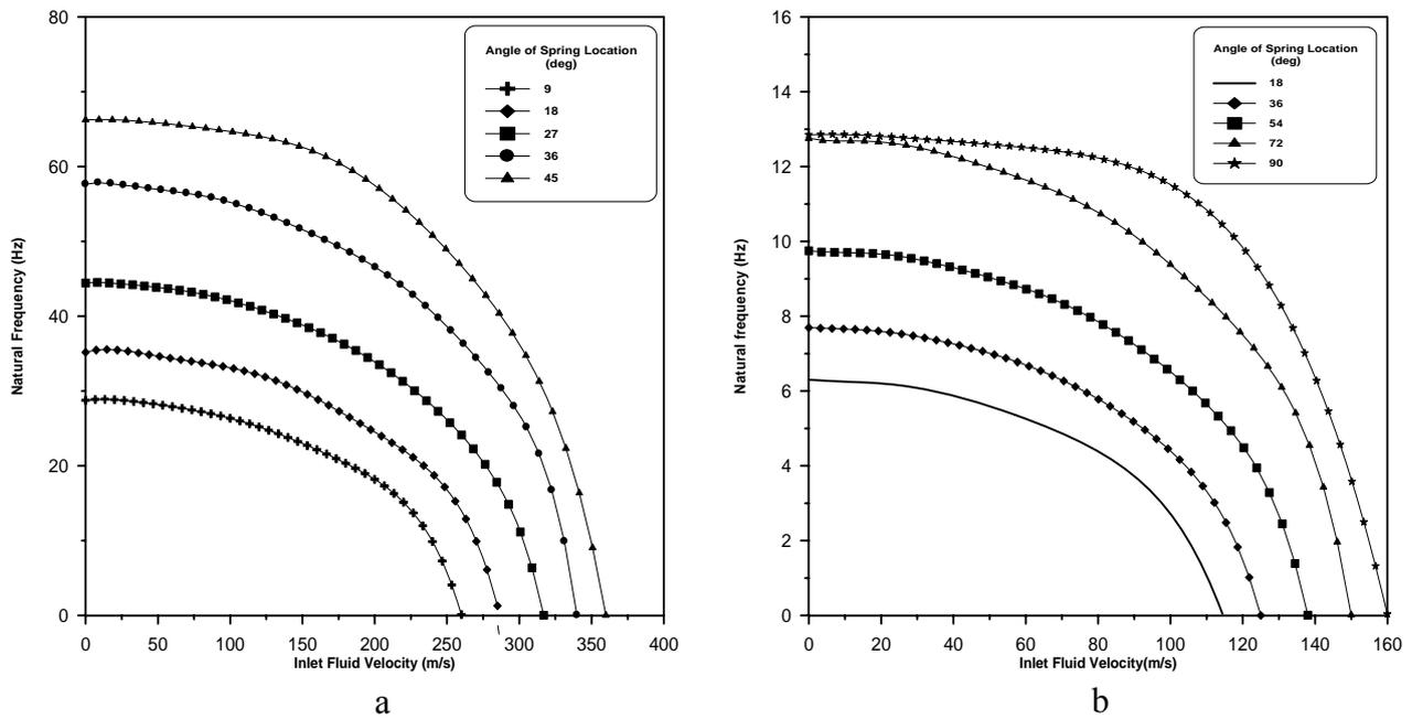
**Fig.(8): Effect the inlet fluid velocity on the natural frequency with varying angle of spring location curved pipe angle ( $a=90^\circ$  and  $b=180^\circ$ )**
