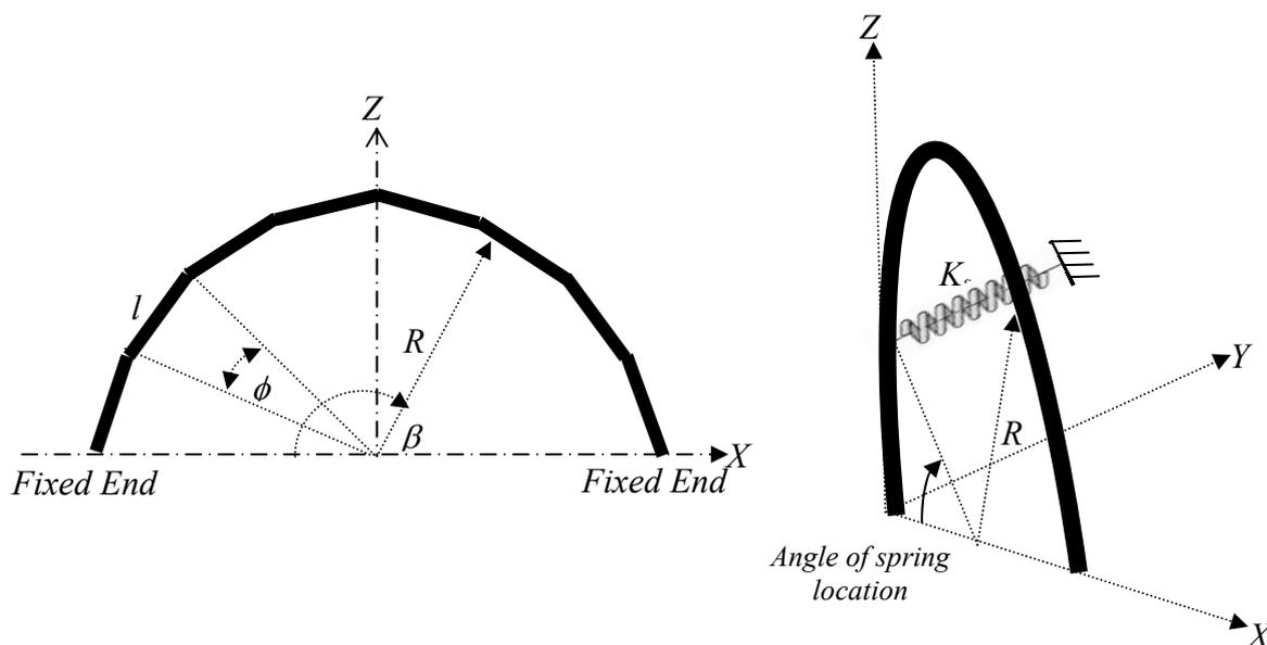
**Fig.(1):** Curved Pipe Model and Angle of Spring Location.
