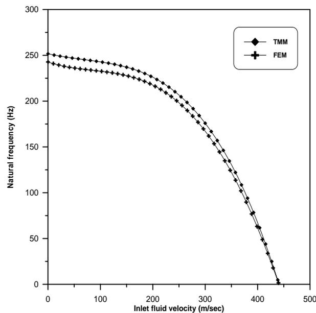
Fig.(5): Effect the inlet fluid velocity on the natural frequency
