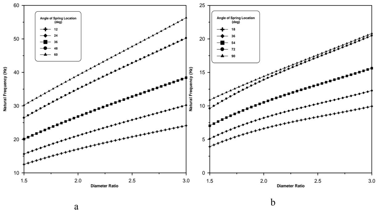
**Fig. (9): Effect the diameter ratio on the natural frequency with varying angle of Spring Location with inlet diameter (ID=3mm) curved pipe angle ( $a=120^\circ$  and  $b=180^\circ$ )**
