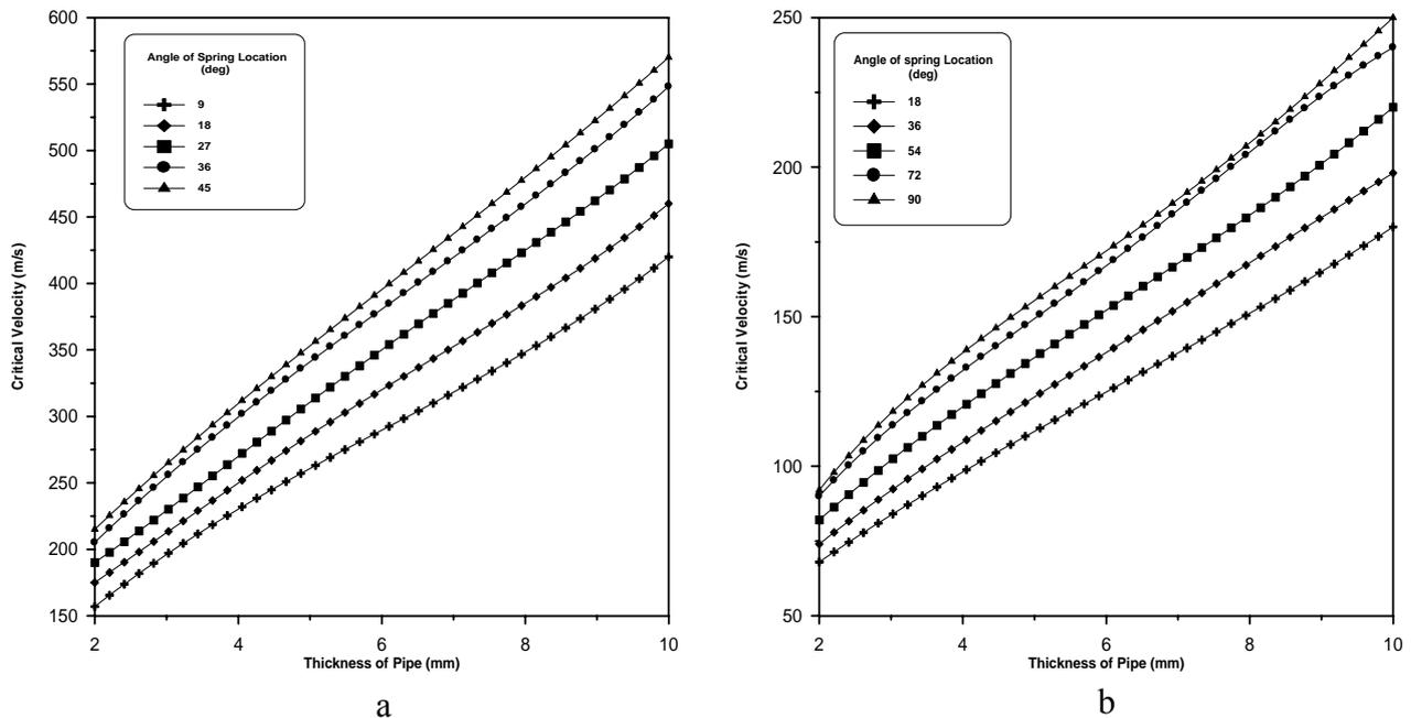
**Fig.(10): Effect the curved pipe thickness on the critical velocity with varying angle of spring location**
