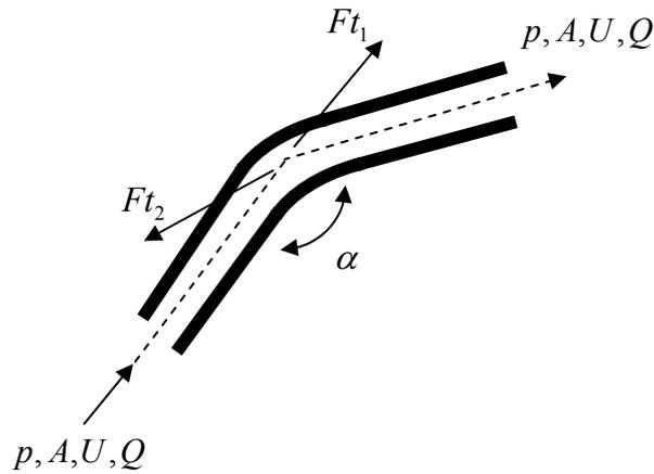
**Fig.(3): Tension forces in curved pipe bend.**
