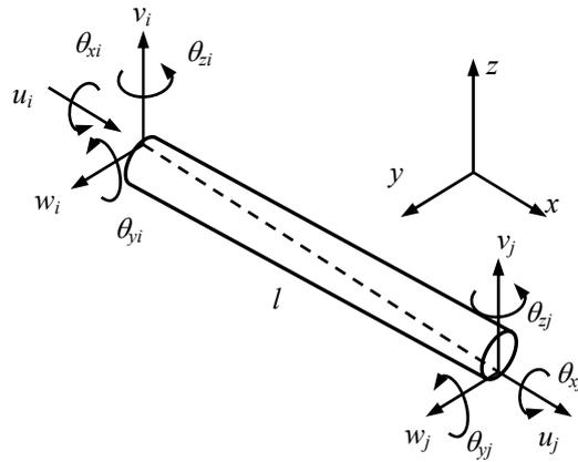
**Fig.(2): Degree of freedom of pipe element.**
