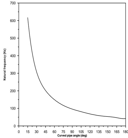
Fig.(4): Effect the curved pipe angle on the natural frequency
