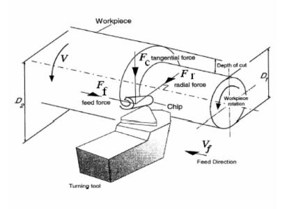
Figure (1) Cutting force components in turning
