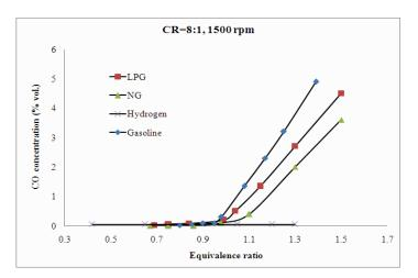
Figure 4, CO concentrations for wide range of equivalence ratios for the four fuels used in research at CR=8:1
