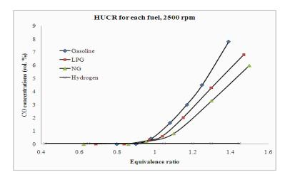
Figure 7, CO concentrations for wide range of equivalence ratios for the four fuels used in research at HUCR for each fuel and 2500 rpm engine speed (high speed)
