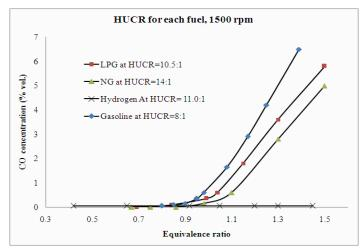
Figure 5, CO concentrations for wide range of equivalence ratios for the four fuels used in research at HUCR for each fuel and 1500 rpm engine speed (medium speed)
