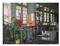
Fig. 1, Recardo engine and its accessories used in this study The following instruments were used for the analysis of the emissions:
