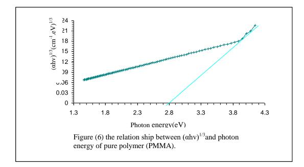
Indirect transition which equals (2.95eV). Figure (7) and figure (8) represent the same relationship but of the polymer filled with(TiO<sub>2</sub>) with volume percentages (40,60) wt.%. In the same way, we can be obtained the value
