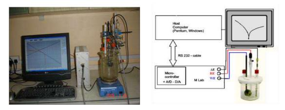
Fig(9)The unit used for electrochemical corrosion.
