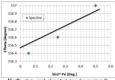
Fig.(8) . photo graph of residual stress for specimen D.
