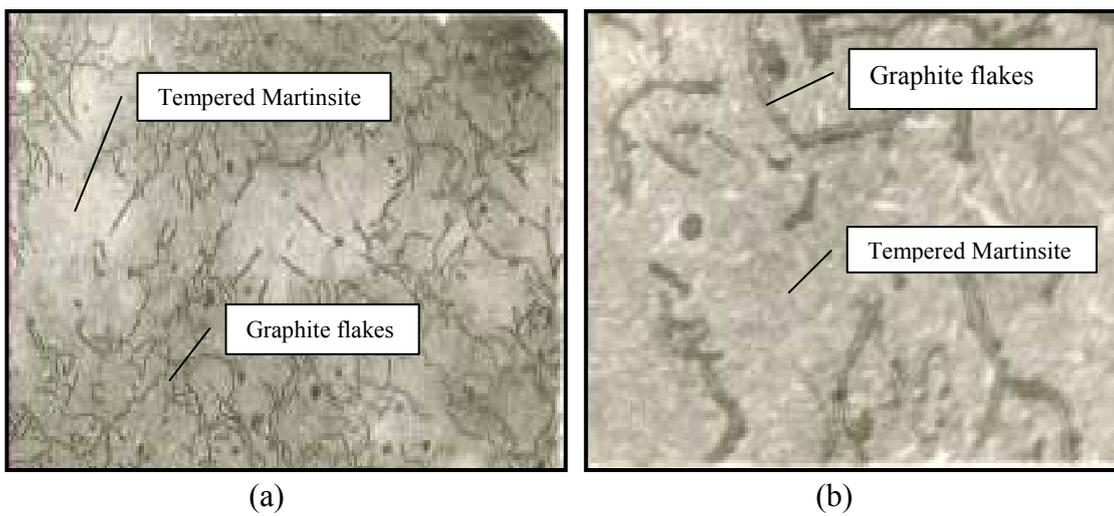
Figure (4.4):Optical microstructure of gray cast iron samples in quenched and tempered conditions: a. 200 X and b. 500 X.
