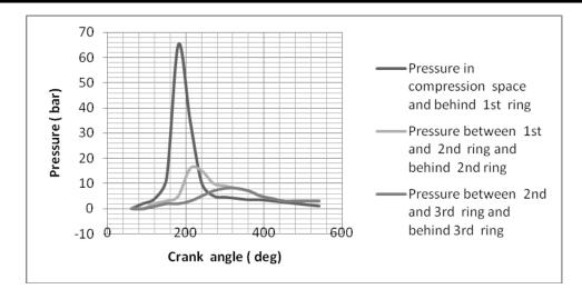
Fig-12. Pressure distribution , case B ,N= 1500 rpm.
