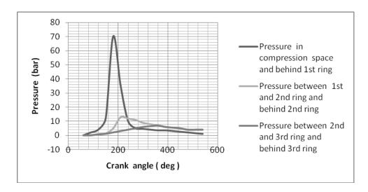
Fig-9. Pressure distribution between and behind piston ring,case A,N=1500 rpm.
