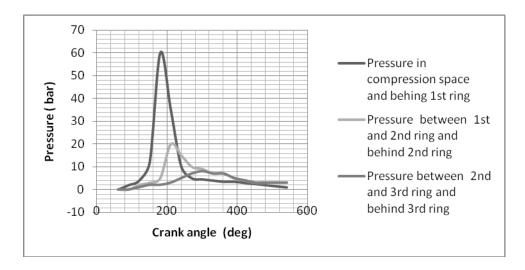
Fig-15. Pressure distribution case -C, N=1500 rpm
