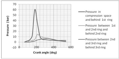
Fig -14. Pressure distribution, case- C, N=1000 rpm.
