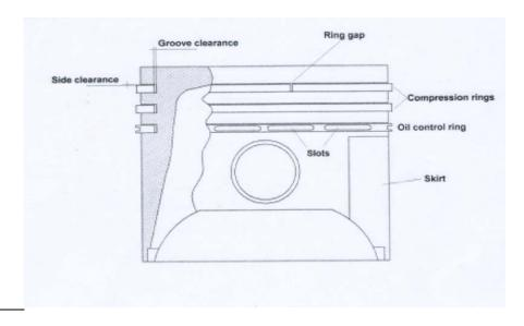
Fig-1. Piston and piston rings
