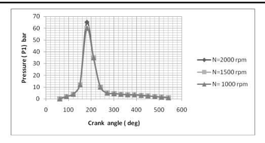
Fig -6. Pressure indicator diagram of as a function of crank angle, case B.
