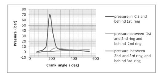
Fig-8. Pressure distribution between and behind piston ring, case A,N=1000
