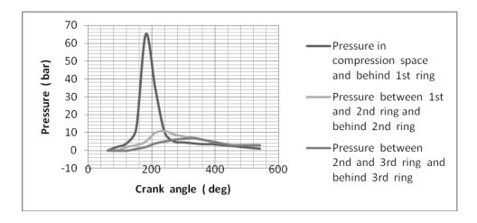
Fig-11.Pressure distribution ,case- B , N= 1000 rpm.
