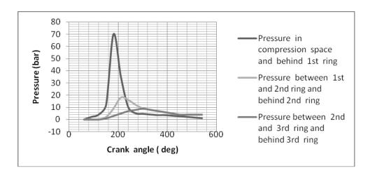
Fig-10.Pressure distribution between and behind piston ring,case-A, N=2000rpm
