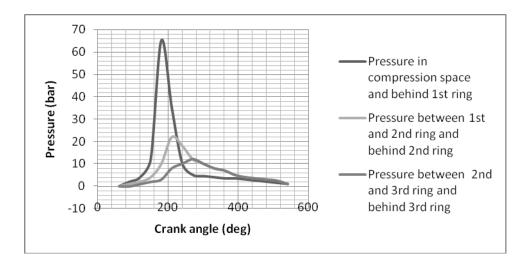
Fig-13. Pressure distribution, case -B, N = 2000 rpm.
