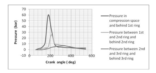
Fig-16 .Pressure distribution case-C ,N= 2000 rpm
