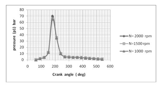
Fig-5. Pressure indicator diagram of as a function of crank angle, case A.
