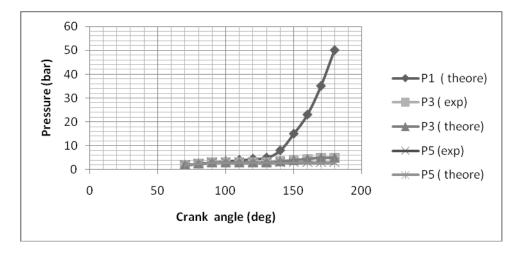
Fig-17. Theoretical and experimental results of pressures inside the inter-ring crevices region P1,P2,P3 as function of crank angle case-C.
