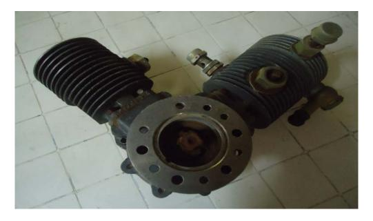
Fig-2. Reciprocating air compressor (V-AK 150)
