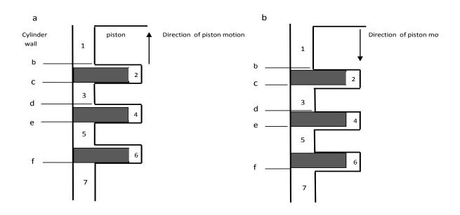
Fig-3. Schmatic diagram for the gas flow through piston rings.
