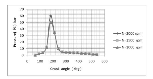
Fig-7. Pressure indicator diagram of as a function of crank angle ,case C.
