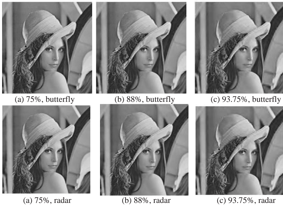
Fig. (8) JPEG compressed embedded Lena image. The compression ratio and the signature image used are indicated below each image. The scale factor used was \alpha=0.05
