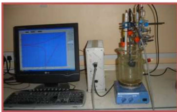
Fig.(2) : Electrochemical corrosion cell used in this study
