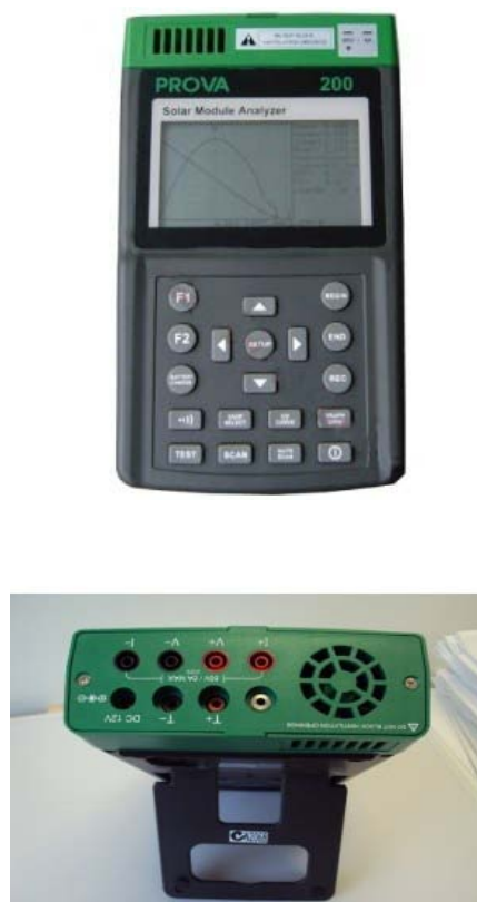
Fig.3: The Prova 200 solar panel analyzer
