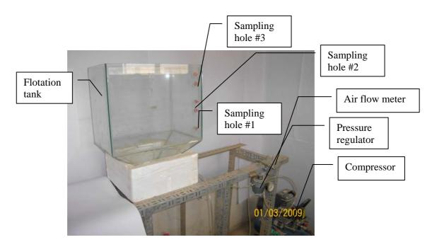
Fig.1. Experimental setup for the Induced Air Flotation System
