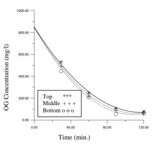
Fig. 13 Oil concentration at the bottom layer vs. time after using 0.5 g/l of Alum as a coagulant for effluent of Dairy Industry
