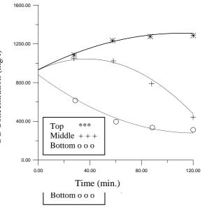
Fig.6 Oil concentration vs. time at different layers of flotation tank and (5 l/min) air flow rate for the effluent of Sweets industry.
