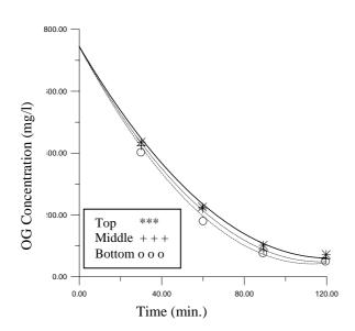
Fig. 12 Oil concentration at the bottom layer vs. time after using 0.5 g/l of Alum as a coagulant for effluent of Sweets Industry
