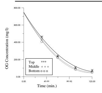
Fig. 10 Oil concentration at the bottom layer vs. time after using 0.4 g/l of Alum as a coagulant for effluent of Sweets Industry
