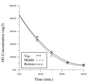
Fig. 11 Oil concentration at the bottom layer vs. time after using 0.4 g/l of Alum as a coagulant for effluent of Dairy Industry
