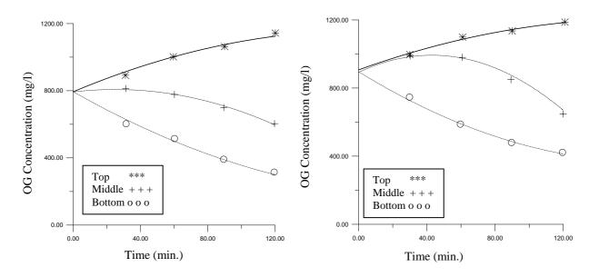
Fig.2 Oil concentration vs. time at different layers of flotation tank and (1 l/min) air flow rate for the effluent of Sweets industry.
