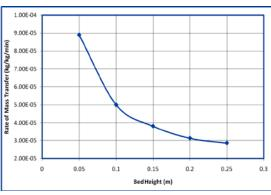
Figure (12): Adsorption rate for different packed heights.
