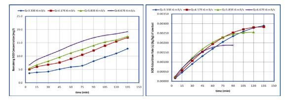
**Figure (6)** breakthrough curves of isothermal adsorption for different influent flow rates.
