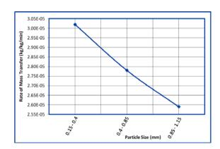
Figure (18) effect of the particle sizes on the rate of mass transfer of BOD<sub>5</sub>.
