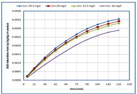
Figure (1): breakthrough curves of isothermal adsorption for different BOD<sub>5</sub> influent initial concentrations.
