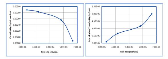
Figure (8): effect of the influent flow rates on the capacity of the sawdust.
