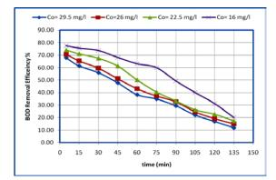
**Figure (5):** effect of the influent initial BOD<sub>5</sub> concentrations on the adsorption removal efficiency of sawdust.
