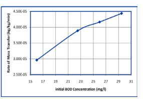
**Figure (3):** effect of the influent initial BOD<sub>5</sub> concentrations on the capacity of the sawdust.
