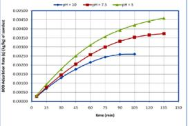
Figure (19): breakthrough curves of isothermal adsorption for different pH of the influent.
