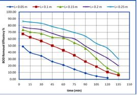
Figure (10): breakthrough curves of isothermal adsorption for different packed heights
