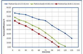
**Figure (15)** the effect of the particle size on the BOD<sub>5</sub> removal efficiency.
