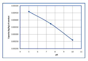
Figure (21): effect of the pH of the influent on the capacity of the sawdust.
