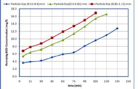
Figure (14) Breakthrough curves of isothermal adsorption for different particle sizes.
