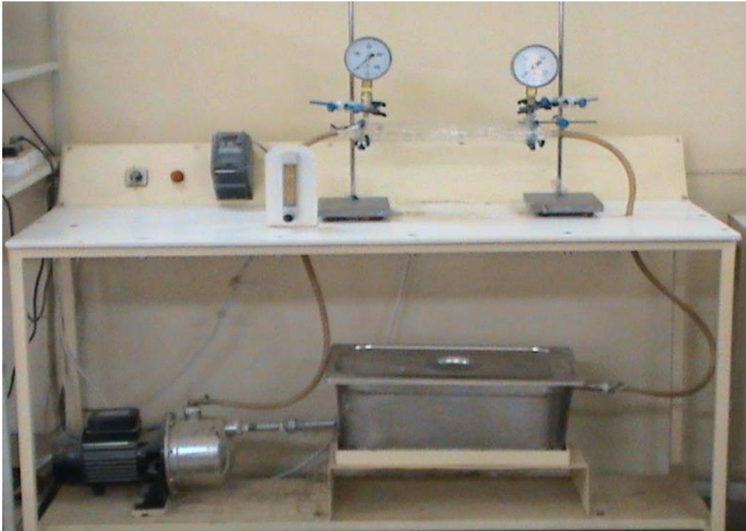
**Fig4 Pressure drop investigation apparatus**
