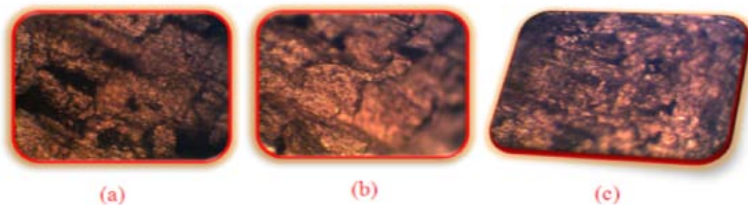
Fig (10) :Micrograph (400 X) of machined surfaces, a cutting speed of 5 m/min and a feed rate of 0.016mm /rev for the alloy sample , (a) S0 where Ra= 4.957, (b) S3 where Ra= 4.32 , (c) SG where Ra= 3.2 \mu m .
