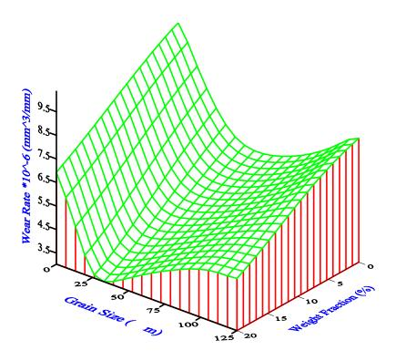
Figure (8): Relationship Between the Grain Size and the Wear Rate of the Polyester Reinforced by (Sio<sub>2</sub>) Particles with Different weight fraction and at Working Conditions (W=4.5 N, V<sub>s</sub>= 2.2 m/sec., and T= 300 Sec.).
