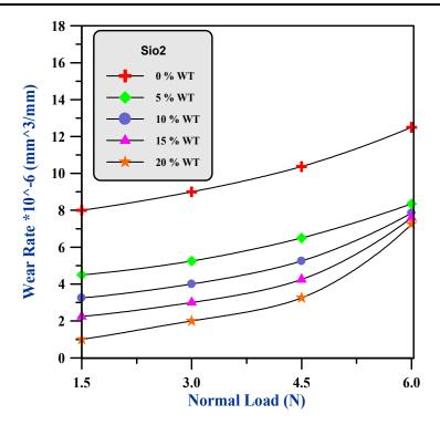
Figure (3): Relationship Between the Normal Load and the Wear Rate of the Polyester Reinforced by (Sio<sub>2</sub>) Particles with Grain Size (25 μm) and Working Conditions (V<sub>s</sub>= 2.2 m/sec., and T= 300 Sec.).
