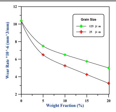
Figure (7): Relationship Between the Weight Fraction and the Wear Rate of the Polyester Reinforced by (Sio<sub>2</sub>) Particles with Different Grain Size and at Working Conditions (W=4.5 N, V<sub>s</sub>= 2.2 m/sec., and T= 300 Sec.).
