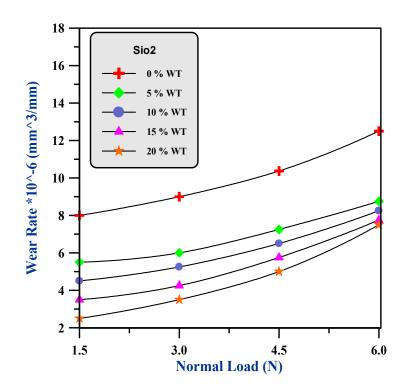
Figure (4): Relationship Between the Normal Load and the Wear Rate of the Polyester Reinforced by (Sio<sub>2</sub>) Particles with Grain Size (125  $\mu$ m) and Working Conditions (V<sub>s</sub>= 2.2 m/sec., and T= 300 Sec.).
