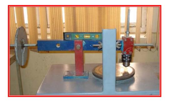
Figure (1): Pin -on- Disc Wear Test Apparatus.
