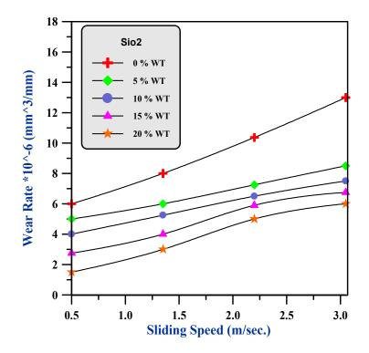
Figure (6): Relationship Between the Sliding Speed and the Wear Rate of the Polyester Reinforced by (Sio<sub>2</sub>) Particles with Grain Size (125 μm) and Working Conditions (W=4.5 N, and T= 300 Sec.).
