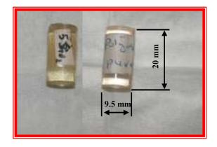
Figure (2): Samples and Dimensions of the test specimens.
