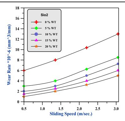
Figure (5): Relationship Between the Sliding Speed and the Wear Rate of the Polyester Reinforced by (Sio<sub>2</sub>) Particles with Grain Size (25 μm) and Working Conditions (W=4.5 N, and T= 300 Sec.).
