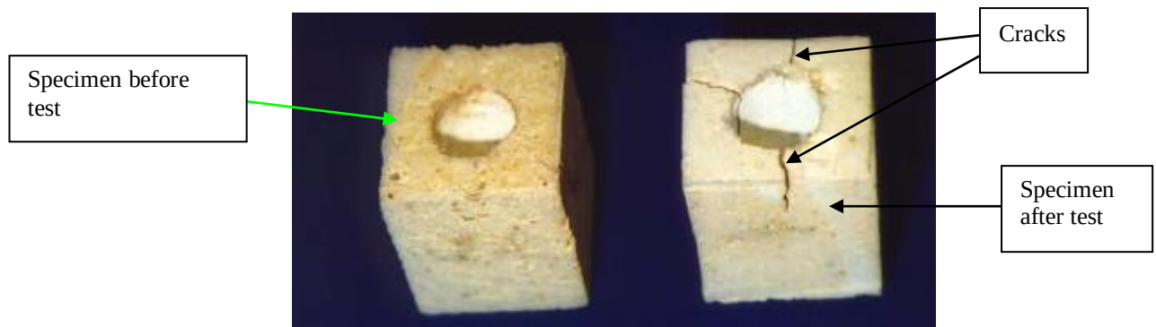
Fig 5: The alkali attack test result in visible cracks caused by volume increasing (High alumina brick).
