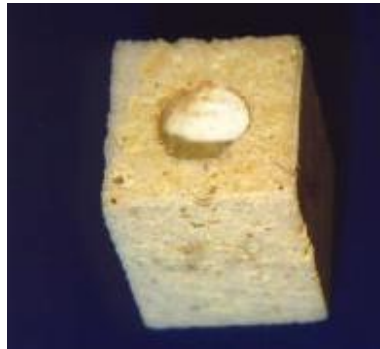
Fig 2: 50 mm length cube specimen with 25 mm diameter half sphere for alkali attack test (high alumina refractory)
