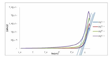
Figure(5) (α hυ)2 (eV/ cm)2 vs. hυ(ev) of In<sub>2</sub>O<sub>3</sub> NPs at different laser power density.
