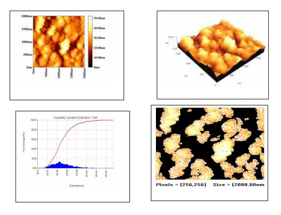
Figure (8) Represents the AFM micrograph of In<sub>2</sub>O<sub>3</sub> films deposited at the highest energy of (400 mj).
