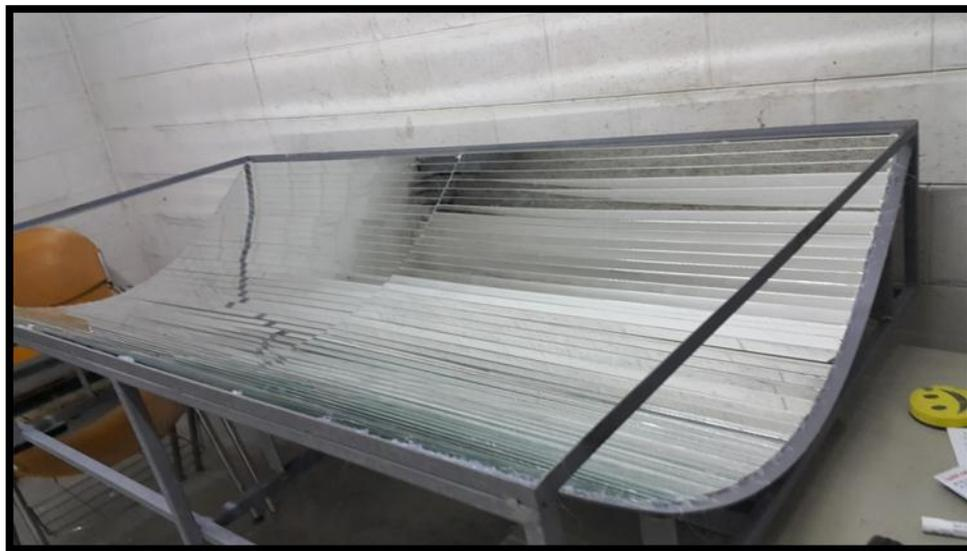
Figure (4 b): Parabolic Reflector which used in the experimental work.
