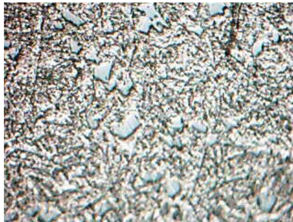
Fig.3 Al-20Si modified by Sr (sample 2) x200
