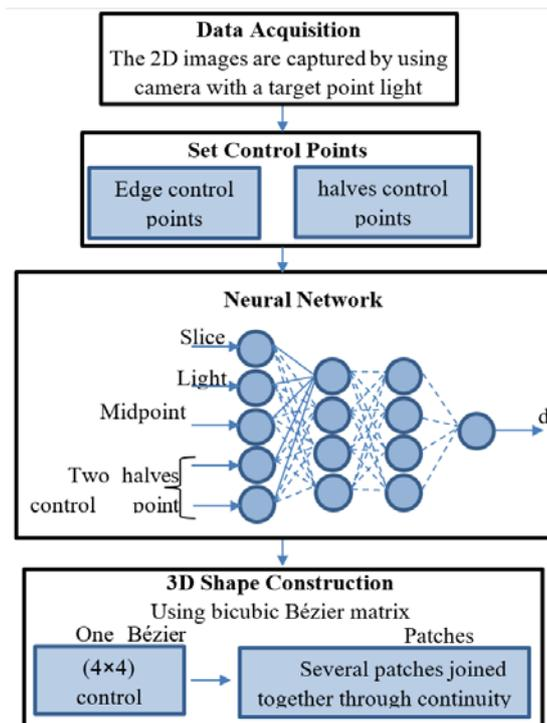
FIG. 7. THE BLOCK DIAGRAM OF THE PROPOSED APPROACH FOR DEPTH ESTIMATION AND SHAPE. RECONSTRUCTION.
