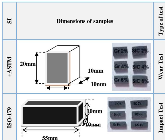
Figure 1. Dimensions of samples
