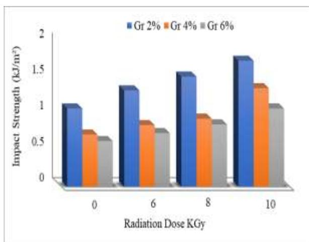
**Figure 4.** Impact strength for Gr-reinforced epoxy with weight fraction after irradiation with different doses of gamma rays.
