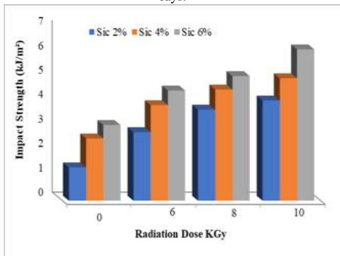
**Figure 5.** Impact strength for SiC-reinforced epoxy with weight fraction after irradiation with different doses of gamma rays.
