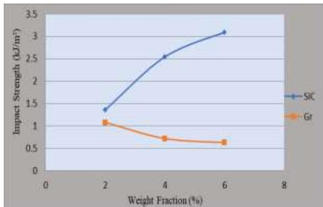
**Figure 3.** Impact strength for SiC-reinforced epoxy & Gr-reinforced epoxy with weight fraction.
