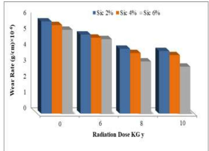
**Figure 8.** Wear rate for SiC-reinforced epoxy with weight fraction after irradiation with different doses of gamma rays
