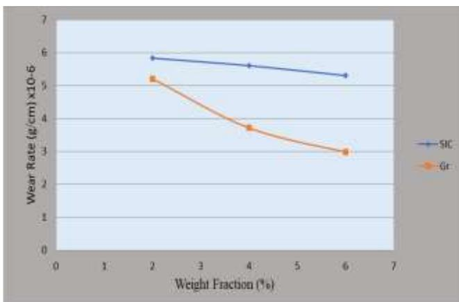
**Figure 6.** Wear rate for Gr-reinforced epoxy & SiC-reinforced epoxy with weight fraction.
