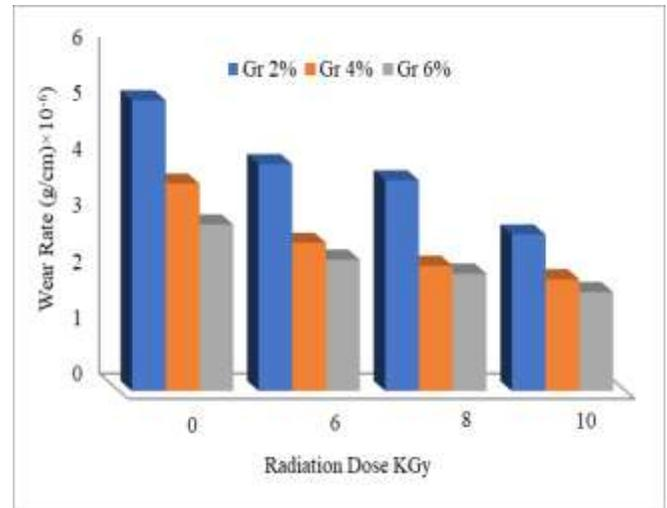
**Figure 7.** Wear rate for Gr-reinforced epoxy with weight fraction after irradiation with different doses of gamma rays
