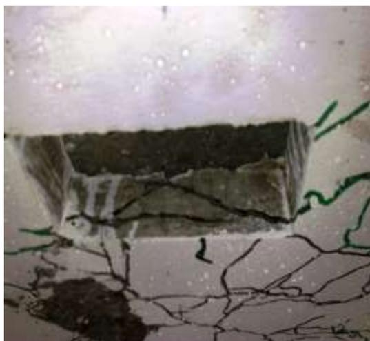
**Fig.(22) Crack Pattern at Failure for Specimen S3 within The Opening.**
