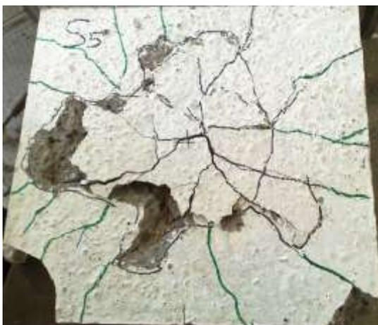
**Fig.(19)Crack Pattern at Failure for Specimen S5.**
