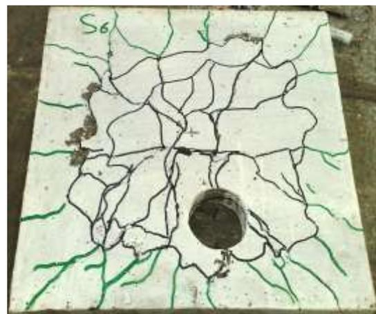
**Fig.(20) Crack Pattern at Failure for Specimen S6.**
