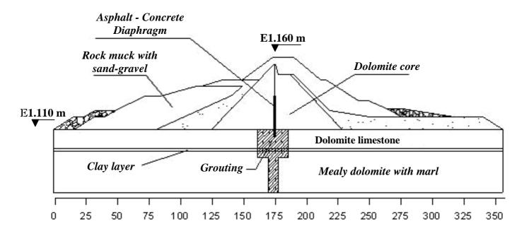
Figure(5): Typical cross section of Haditha Dam with ground profile The zoned embankment and the ground physical mechanics parameters are presented in table 2.
