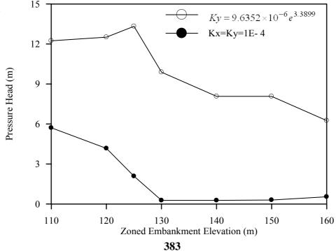
Figure(9):Influence of variation of permeability on pressure heads distribution in section (3 - 3) for various dam levels in the D/S face.
