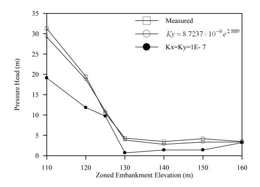
Figure(8):Influence of variation of permeability on pressure heads distribution in section (2 - 2) for various dam levels in the central core.
