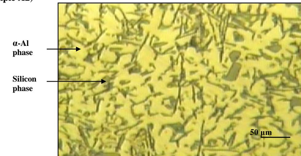
**Fig.6** The microstructure of squeeze cast sample at a applied pressure 38 MPa ( sample A3)
