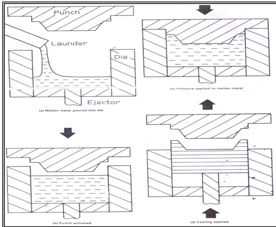
Fig. 2 Direct squeeze die casting process [10].
