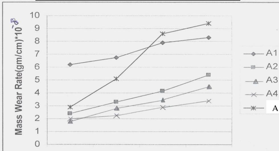
Fig.8 Effect of applied load in wear rate for squeeze cast samples of alloy (Al-12%Si) which are produced at different casting pressures, at a sliding speed of 2.7m/sec and sliding time of 20min during wear test
