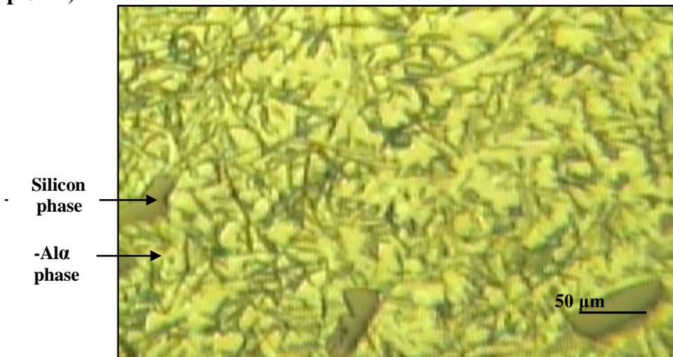
**Fig.5** The microstructure of squeeze cast sample at a applied pressure 23 MPa ( sample A2)
