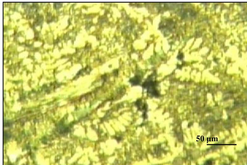
Fig.3 The microstructure of gravity die cast sample ( sample A)
