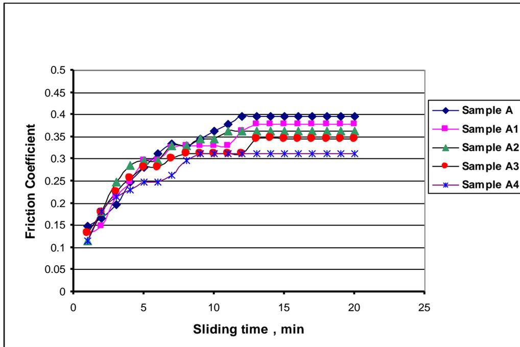
**Fig.9** The effect of sliding time in the friction coefficient ( $\mu$ ) for squeeze cast samples of alloy (Al-12%Si) which are produced at different casting pressures, at a sliding speed of 2.7m/sec , applied load of 20N and sliding time of 20min during wear test
