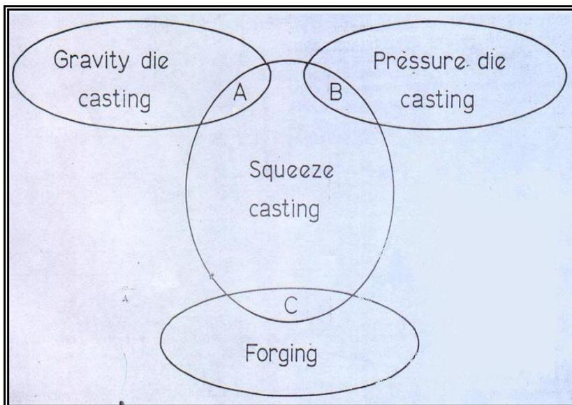
**Fig. 1** Squeeze die casting process as a combined process of gravity die casting, pressure die casting and forging processes [8]
