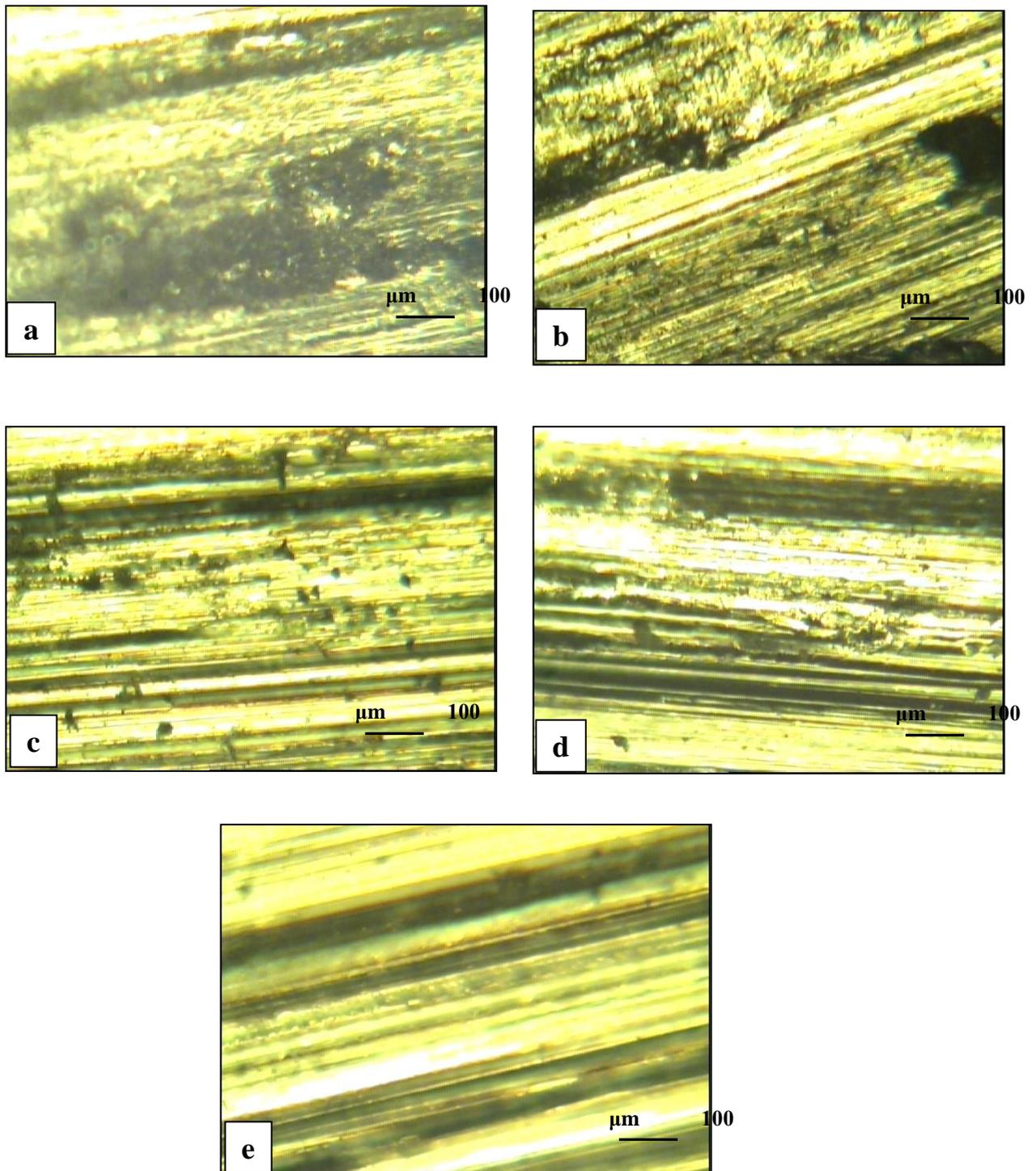
**Fig.11** Micrographs of the worn surfaces of the alloy(Al-12%Si) at a sliding speed of 2.7m/sec , load of 20N and sliding time of 20min
