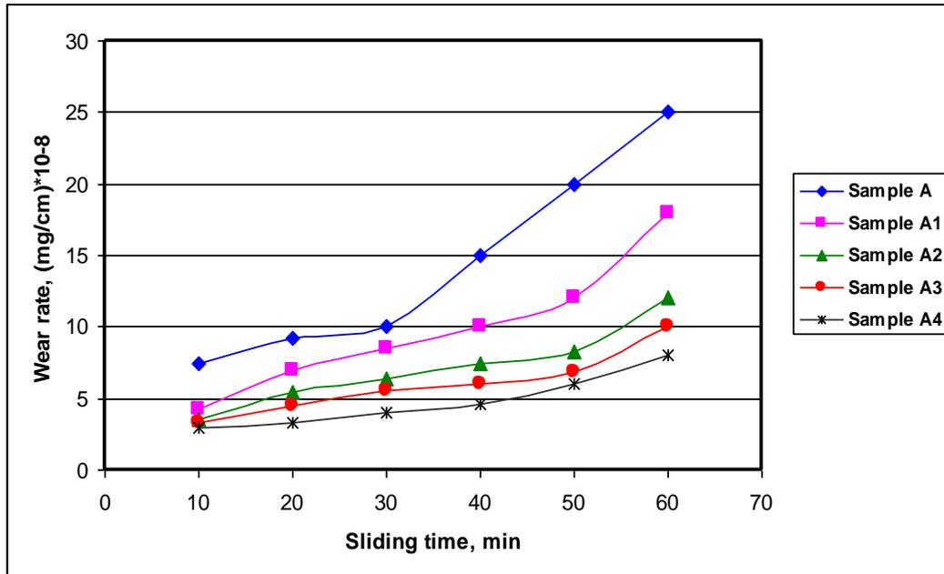
**Fig.10** The effect of sliding time in the wear rate for squeeze cast samples of alloy (Al-12%Si) which are produced at different casting pressures, at a sliding speed of 2.7m/sec and applied load of 20N during wear test
