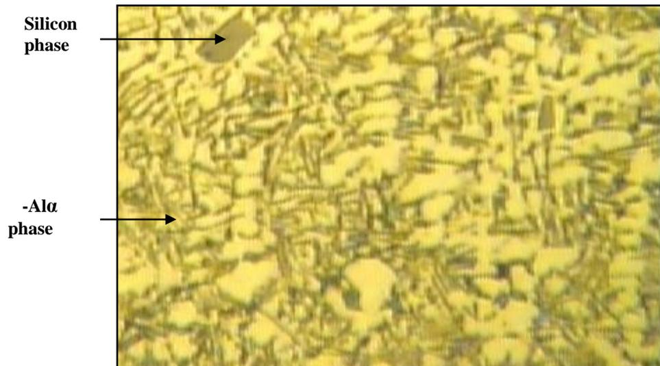
**Fig.4** The microstructure of squeeze cast sample at a applied pressure 7.5MPa ( sample A1)
