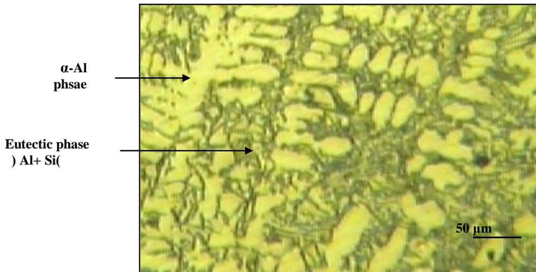
Fig.7 The microstructure of squeeze cast sample at a applied pressure 53 MPa ( sample A4)
