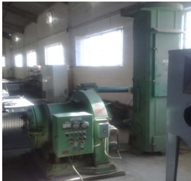
( Fig. 3 ) Shot peening device .
