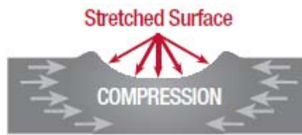
(Fig. 2) Compression resist fatigue cracking [Jack Champaigne 2001 ]
