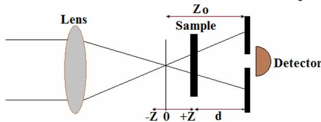
Fig. 3. Z - scan experimental setup.
