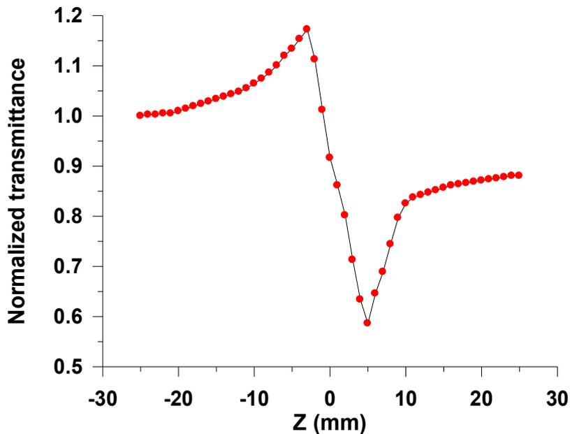
**Fig. 4. Closed aperture Z-scan data for congo red dye when the concentration of the solution is 0.05 mM at 1 mm thickness.**
