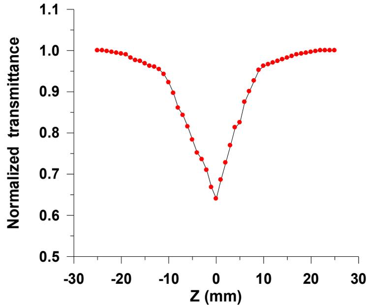
**Fig. 5. Open aperture Z-scan data for congo red dye when the concentration of the solution is 0.05 mM at 1 mm thickness.**
