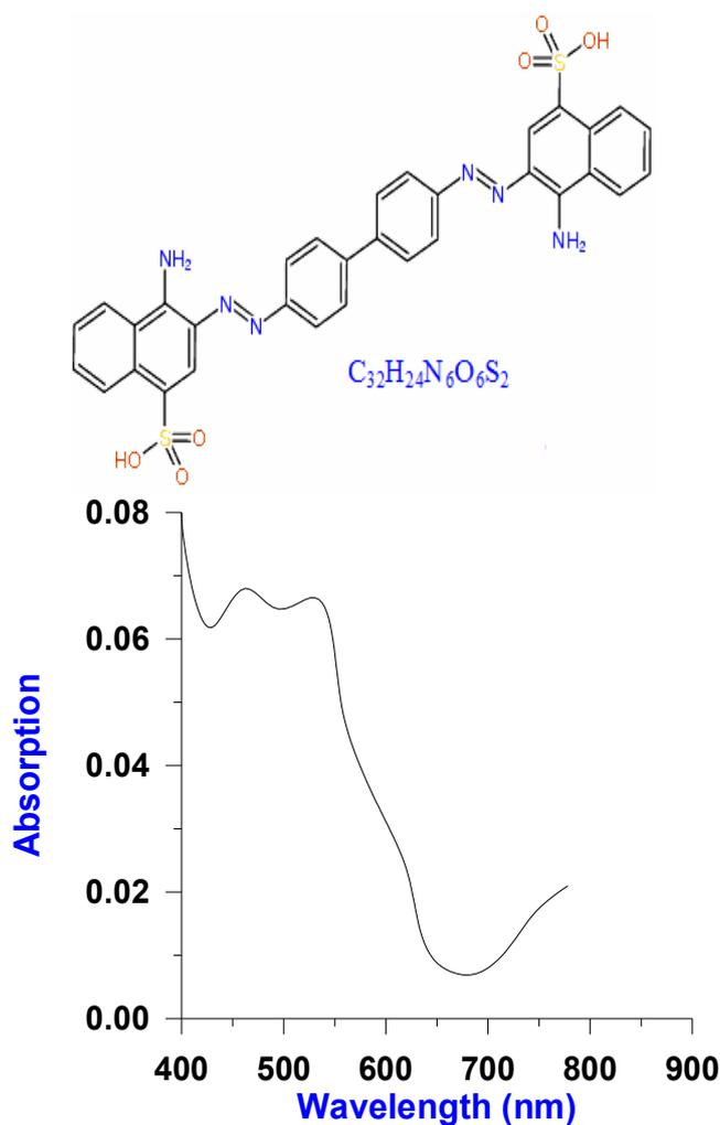
Fig. 1. The molecular structure of the congo red dye[9].
