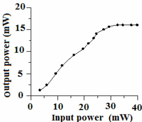
**Fig.7. The nonlinear transmission behavior of congo red dye of 0.05 mM concentration (1mm thickness).**
