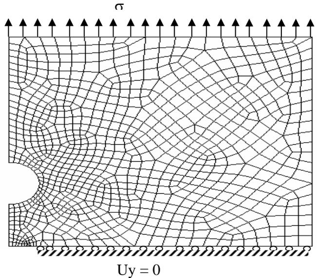
Fig.(5) FE meshes of half plate
