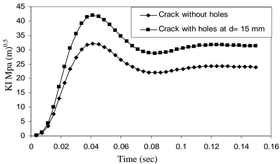
Fig.(18) variation of stress intensity factor with time (s) with central crack
