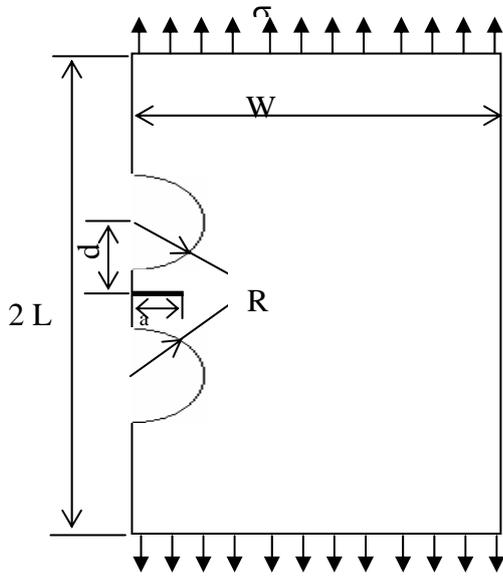
Fig.(4) geometry and loading for plate
