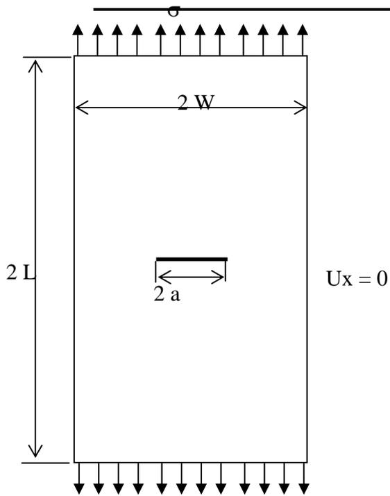
Fig.(8) geometry and loading for plate
