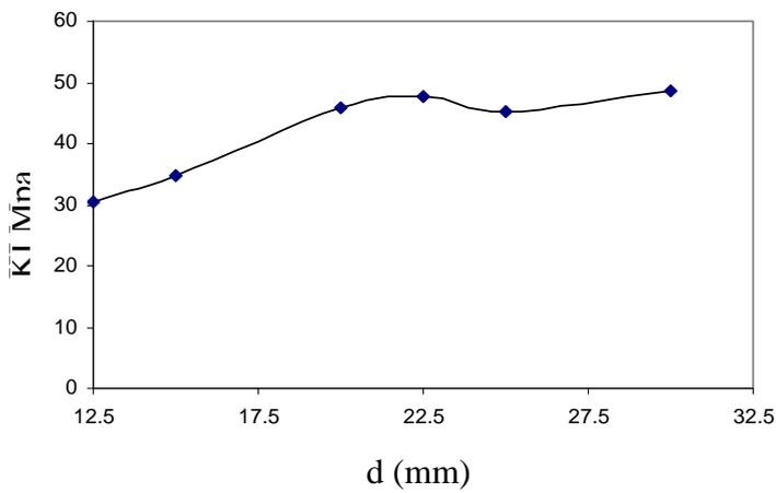
Fig.(14) variation of stress intensity factor with the distant of the auxiliary hole in plate with end crack
