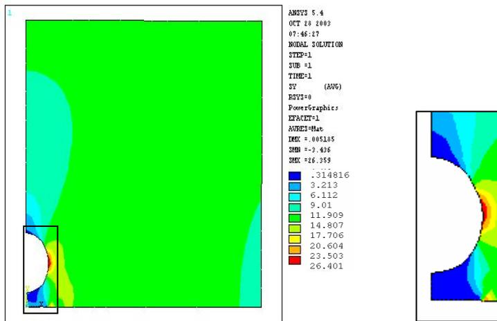
Fig.(13) the reduction of stresses around the crack
