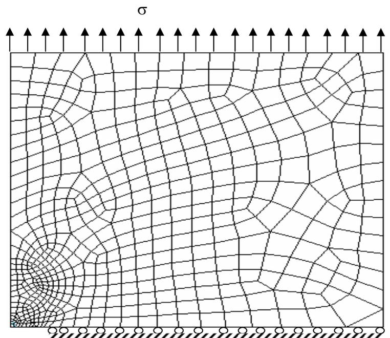
Fig.(2) geometry and loading for plate
