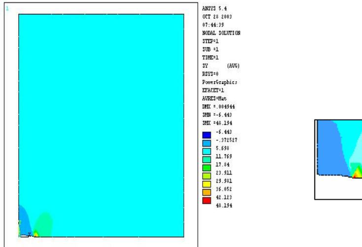
Fig.(12) stresses contour around the crack
