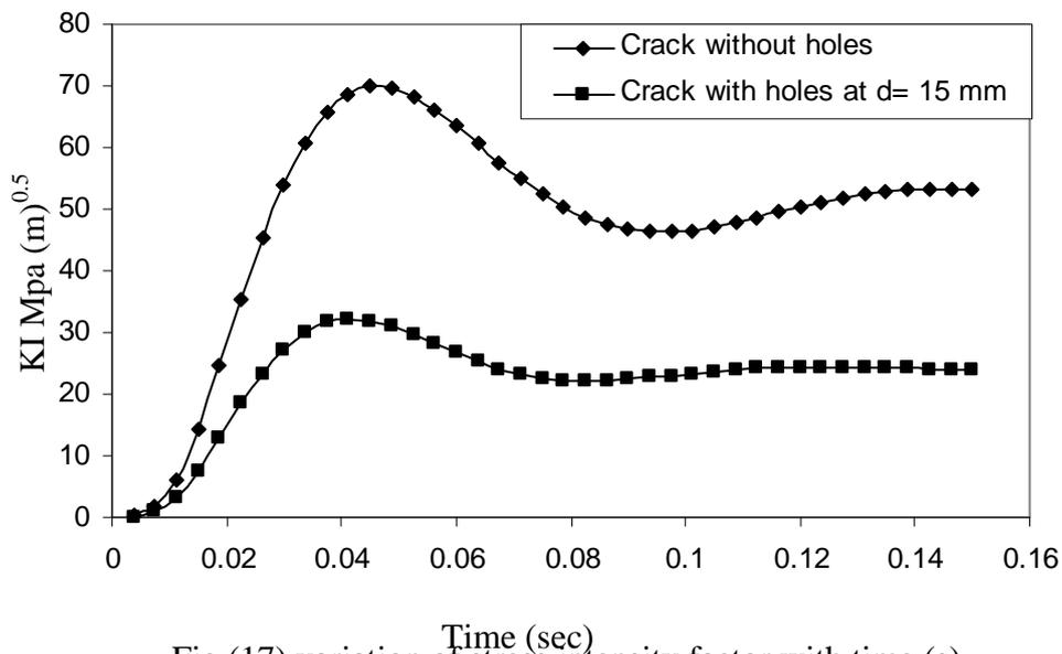
Fig.(17) variation of stress intensity factor with time (s) with end crack
