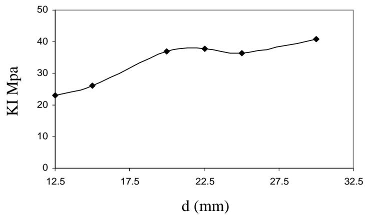
Fig.(15) variation of stress intensity factor with the distant of the auxiliary hole in plate with central crack
