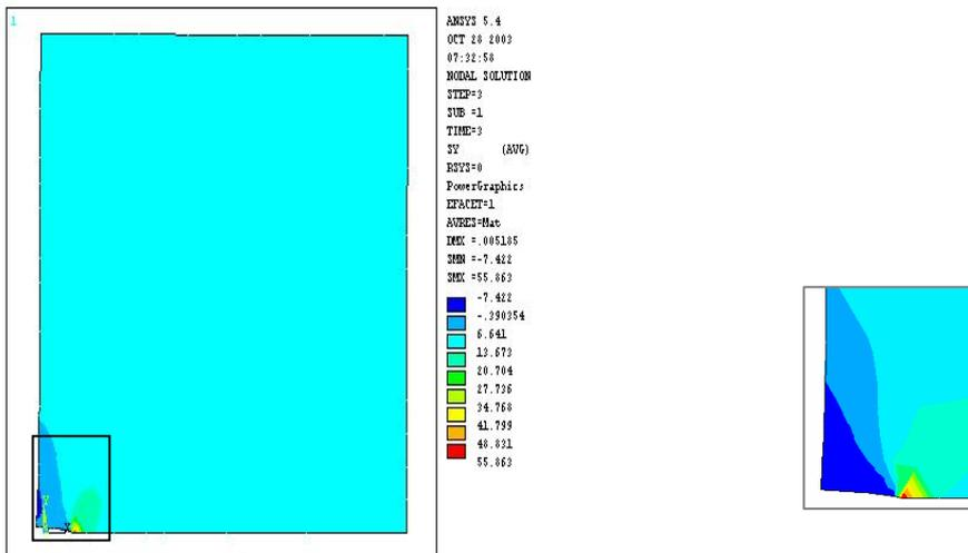
Fig.(6) stresses contour around the crack
