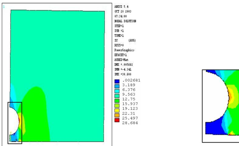
Fig.(7) the reduction of stresses around the crack
