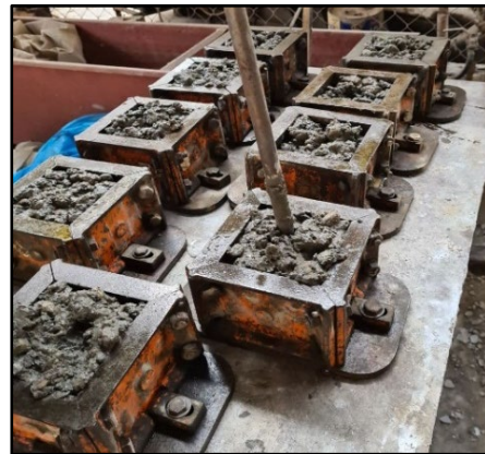
Plate 2: Casting operation of concrete samples
