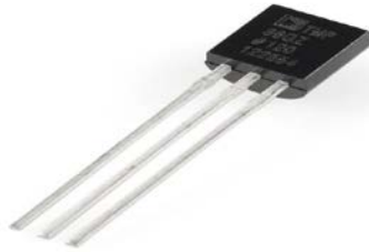
FIG. 4. TEMPERATURE SENSOR TMP36.
