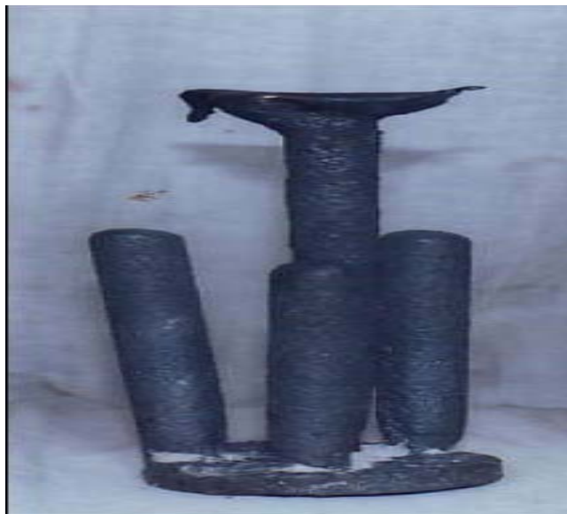
Figure 2 sample of 16 % Ni cast steel produced by sand casting
