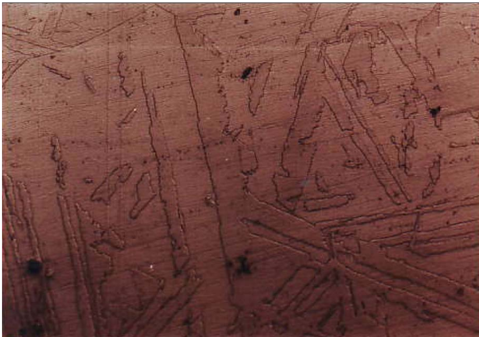
Fig.5. Microstructure produced by annealing 1 hr at 1250C. 100% bcc phase. Etchant 50ccHcl, 25cc HNO 3 , 1g CuCl 2 , 150cc H 2 O X200.
