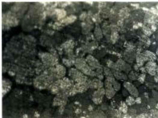
Fig. (6): Effect of smelting conditions on crystal structure of tin, when heating rate, temperature and residence time are equal to 12 °C /min, 443 °C and 0.42 h , respectively.
