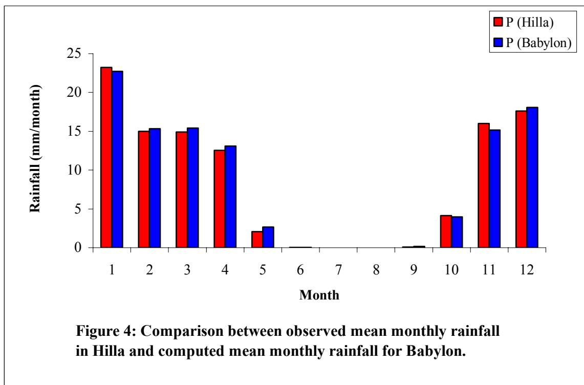
**Figure 4: Comparison between observed mean monthly rainfall in Hilla and computed mean monthly rainfall for Babylon.**
