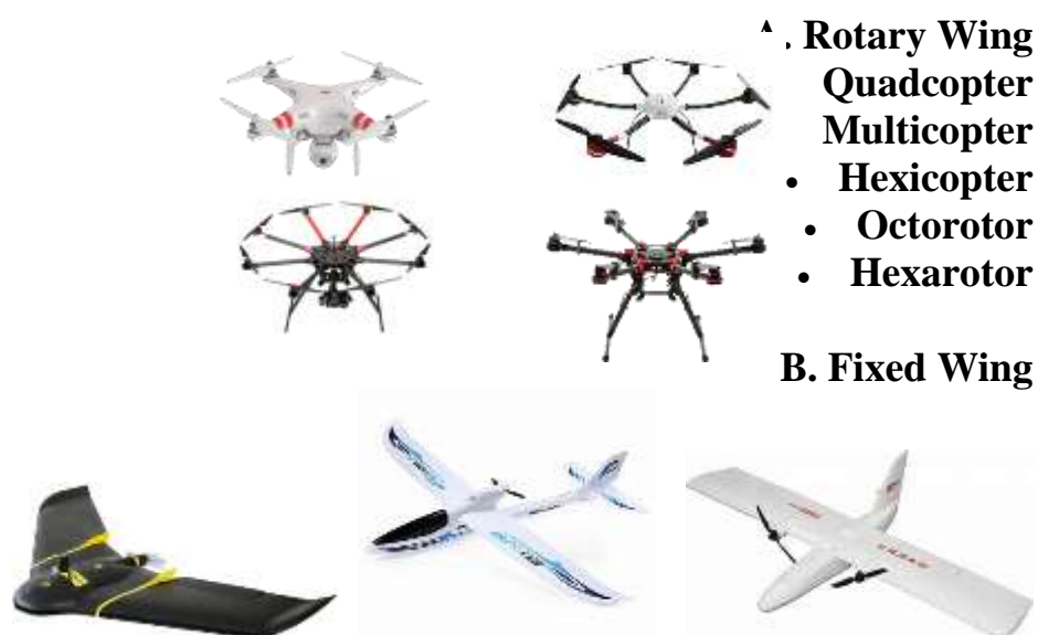
Fig. 2: low-level aerial platforms shapes and names, A: Rotary Wing, B: Fixd Wing.
