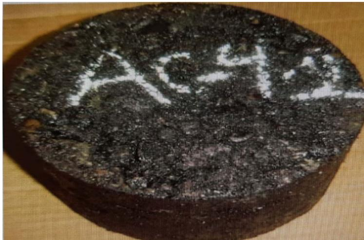
**Figure 1:** Specimen compacted by Superpave Gyratory compactor (Abed, 2010)
