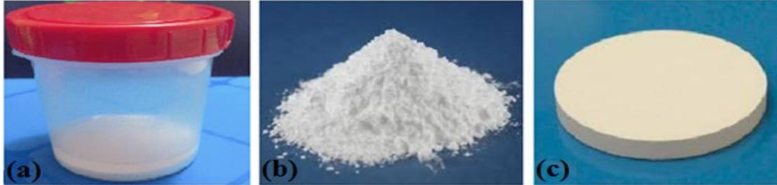
FIG. 1. LITHIUM NIOBATE  $\text{LiNbO}_3$ : A- AFTER THE DRYING PROCESS. B- POWDER. C- TARGET.
