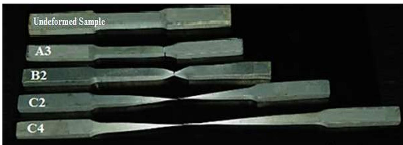
Fig. 1 Fracture of the tensile test samples
