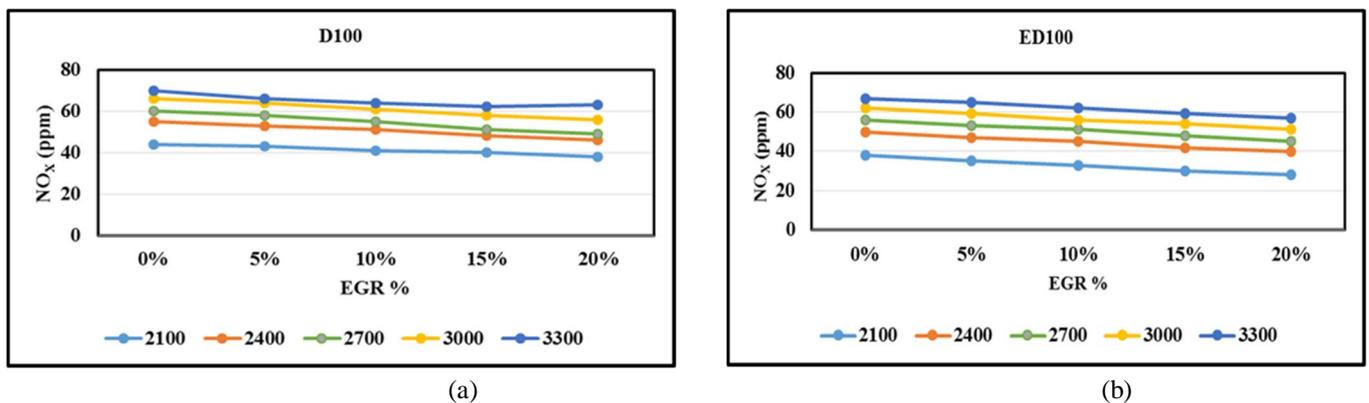
**Figure 5:** (a) The variation of  $\text{NO}_x$  of Iraqi diesel with the different EGR ratios and speed (b) The variation of  $\text{NO}_x$  of Euro diesel with the different EGR ratios and speed
