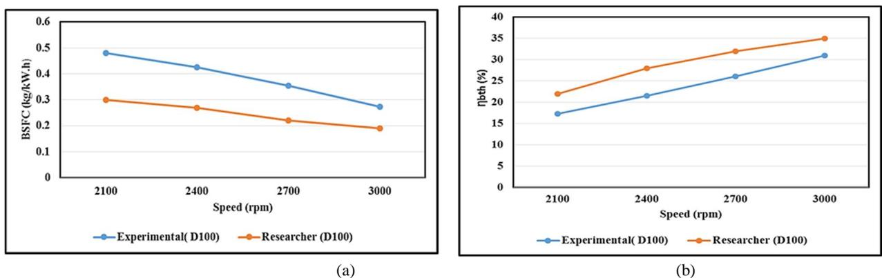
Figure 8: (a). The variation of BSFC at different engine speeds (b)The variation of BTE at different engine speeds
