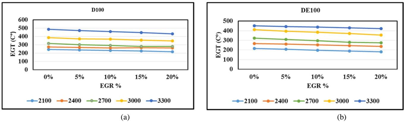
**Figure 4:** (a) The variation of EGT of Iraqi diesel with the different EGR ratios and speed (b) the variation of EGT of Euro diesel with the different EGR ratios and speed
