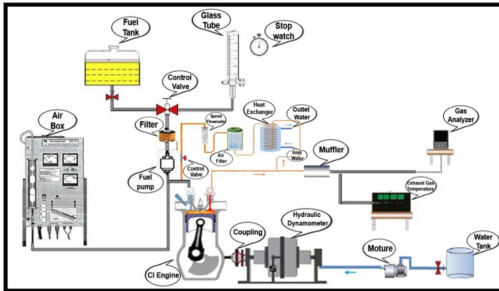
Figure 1: The schematic diagram of the test rig
