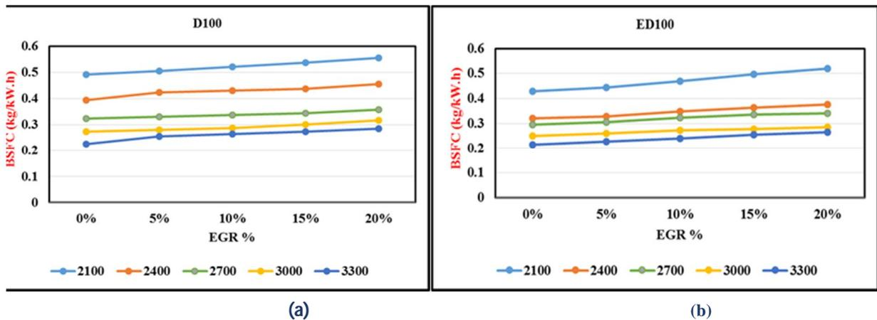
Figure 2: (a) The variation of BSFC of Iraqi diesel with the different EGR ratios and (b) The variation of BSFC of Euro diesel with the different EGR ratios and speed
