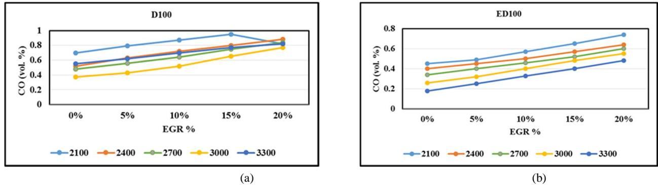
Figure 7: (a).The variation of CO of Iraqi diesel with the different EGR ratios and speed (b) The variation of CO of Euro diesel with the different EGR ratios and speed
