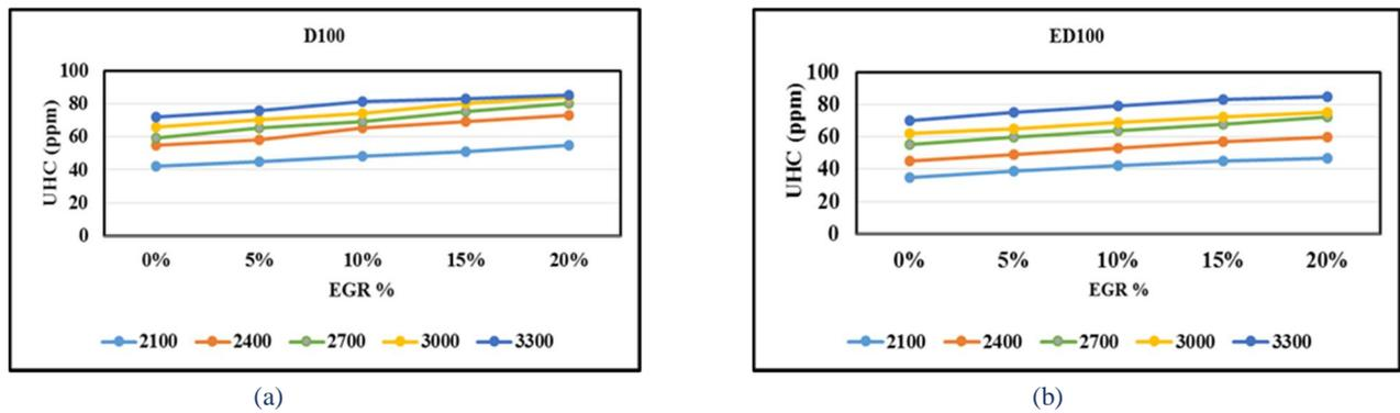
Figure 6: (a). The variation of UHC of Iraqi diesel with the different EGR ratios and speed (b) The variation of UHC of Euro diesel with the different EGR ratios and speed
