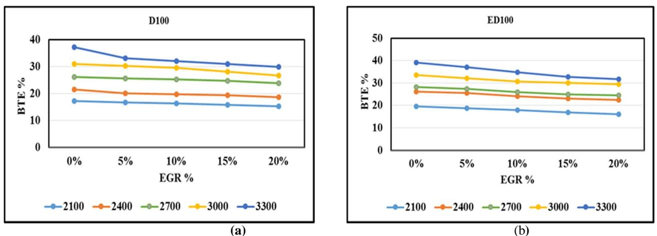
Figure 3: (a). The variation of BTE of Iraqi diesel with the different EGR ratios and speed (b) The variation of BTE of Euro diesel with the different EGR ratios and speed
