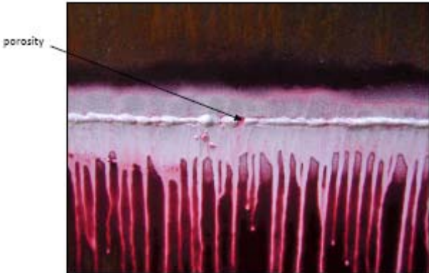
Fig ( 9 )Welding defects- porosity-spatter -roughness
