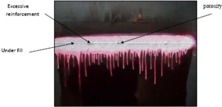
Fig ( 6 ) welding defects – porosity-excessive reinforcement-under fill.
