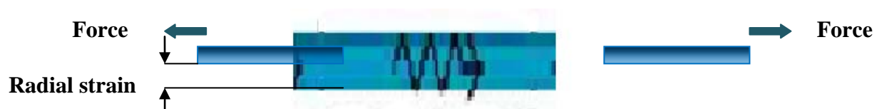
Fig.6.Illustration applying force on an arm of the EOM
